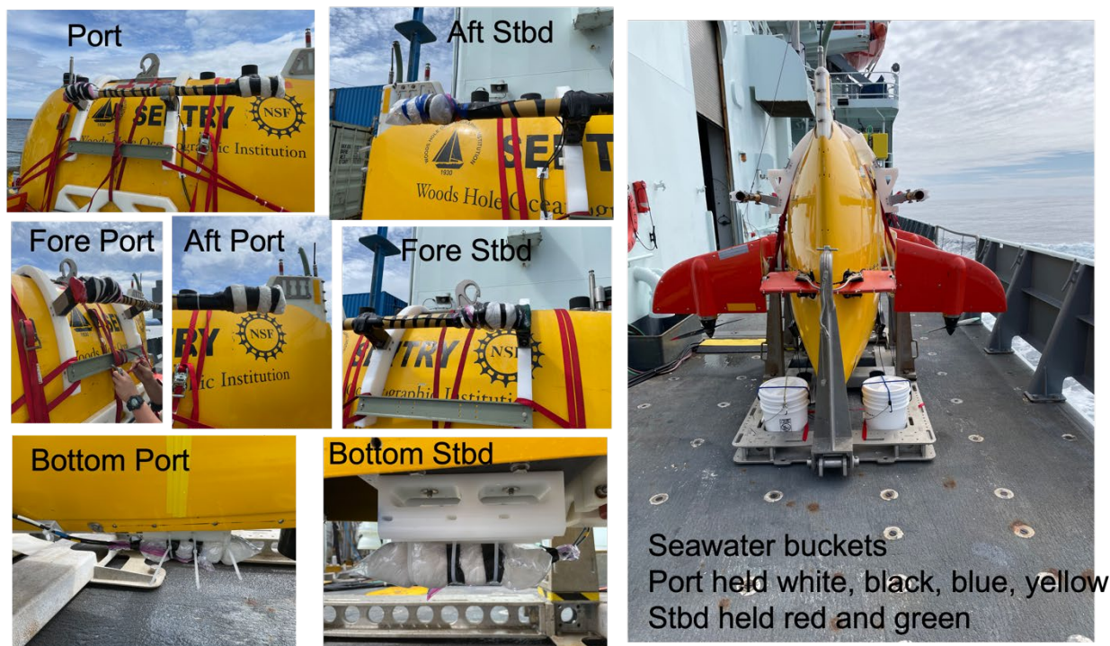
Figure 1 Schematic of the electrode configuration on the Sentry AUV, channel (ch) 0, 1 are crossline and ch 2 and 3 are inline, while ch 4 and 5 are the quasi vertical channels.
