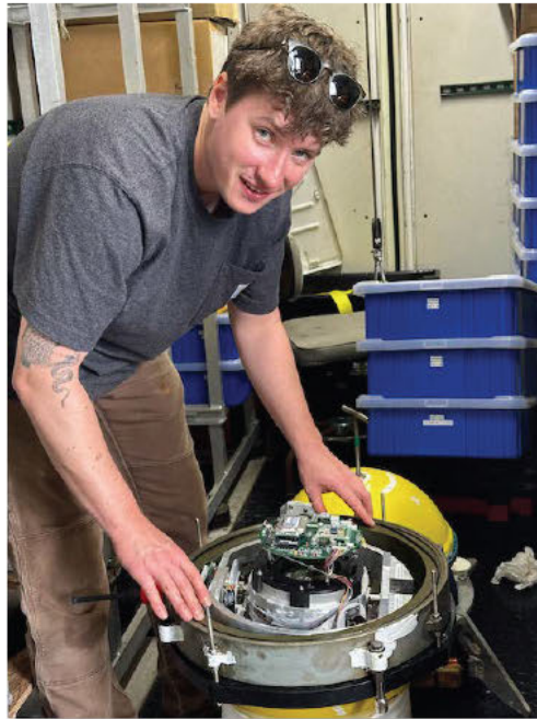
Gavin McCarthy (OBSIC, WHOI) servicing O-ring on seismometer package.
