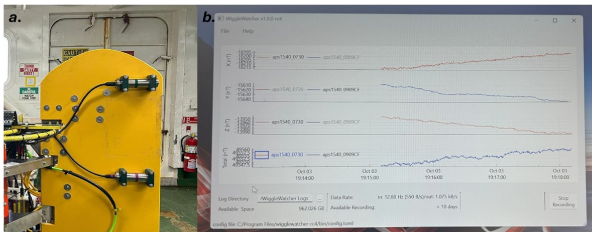
Figure 6.7: (a) APS1540 magnetometers mounted on the TowCam fin, .5 m apart and (b) WiggleWatcher App displaying live magnetometry data for x, y, and z axes, and total field measurement
