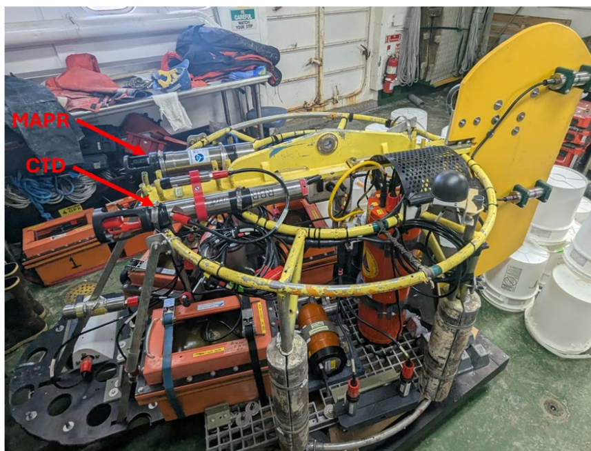
Figure 6.8: MAPR and CTD mounted on the TowCam in forward-facing positions
