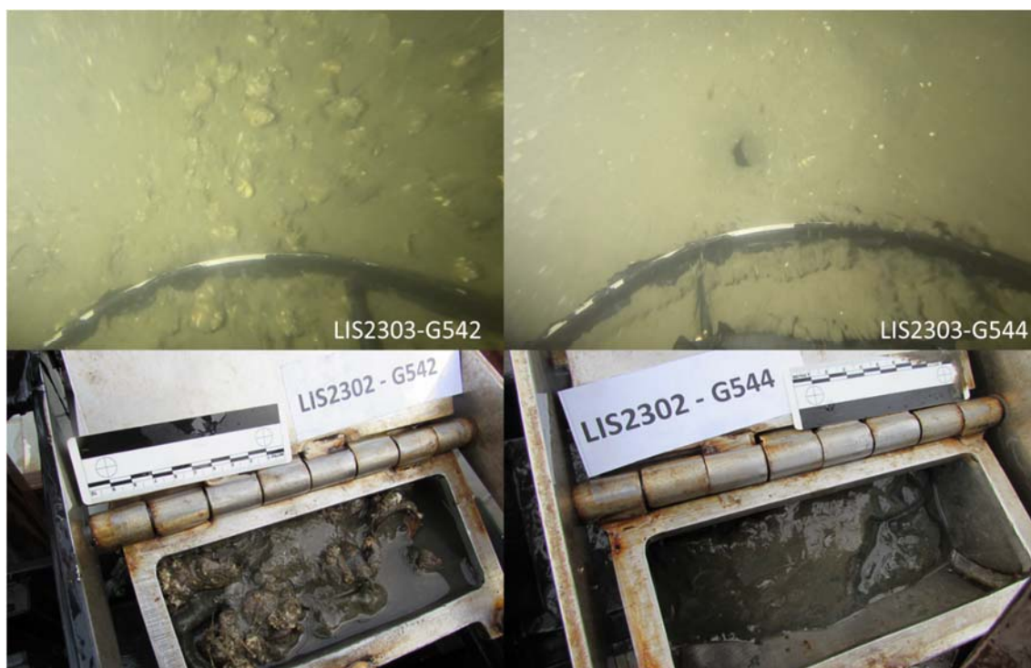
Fig. 4.3: examples of sediment grab bottom images taken by the GoPro system (top) and the corresponding surface grab photos.
