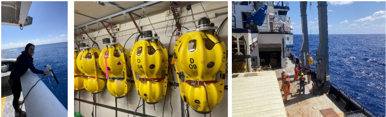
Figure 4.4. A) XBT launch. B) D2 OBS from Woods Hole Oceanographic Institution. C) A D2 OBS is brought back on deck.
