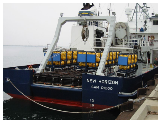
Figure A2.2. A) A LCHEAPO four-component short-period OBS on the seafloor. B) Instruments stacked on the back deck of the R/V New Horizon .
