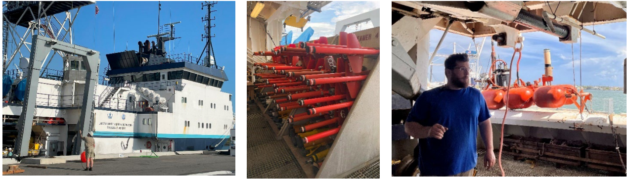
Figure 5.2. A) Langseth at the dock in Port Canaveral. B) A rack with digi-birds ready for deployment. C) Science Officer Cody Bahlau explains the upcoming streamer work, while the tailbuoy is waiting to go overboard.
