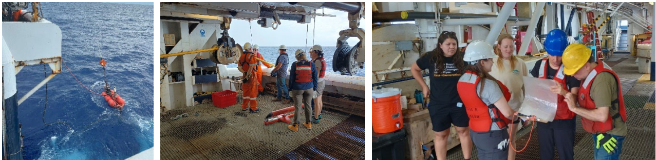
Figure 5.3. A) Tail buoy goes into the water. B) The digi-bird on the deck is ready to be attached to the streamer. C) Shift change on the streamer deck. The check sheet shows which streamer sections and digi-birds have been deployed.
