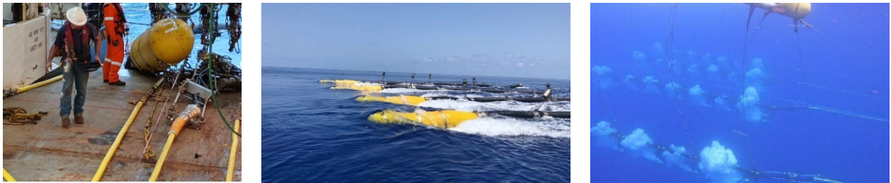
Figure 5.4. A) Mechanics at work on the gun deck. Deployment of the last air-gun float. B) View of the deployed air guns from the work boat. C) Air guns firing underwater.
