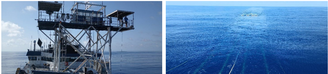
Figure 5.5. A) PSO tower. B) The air guns are firing on a quiet morning.
