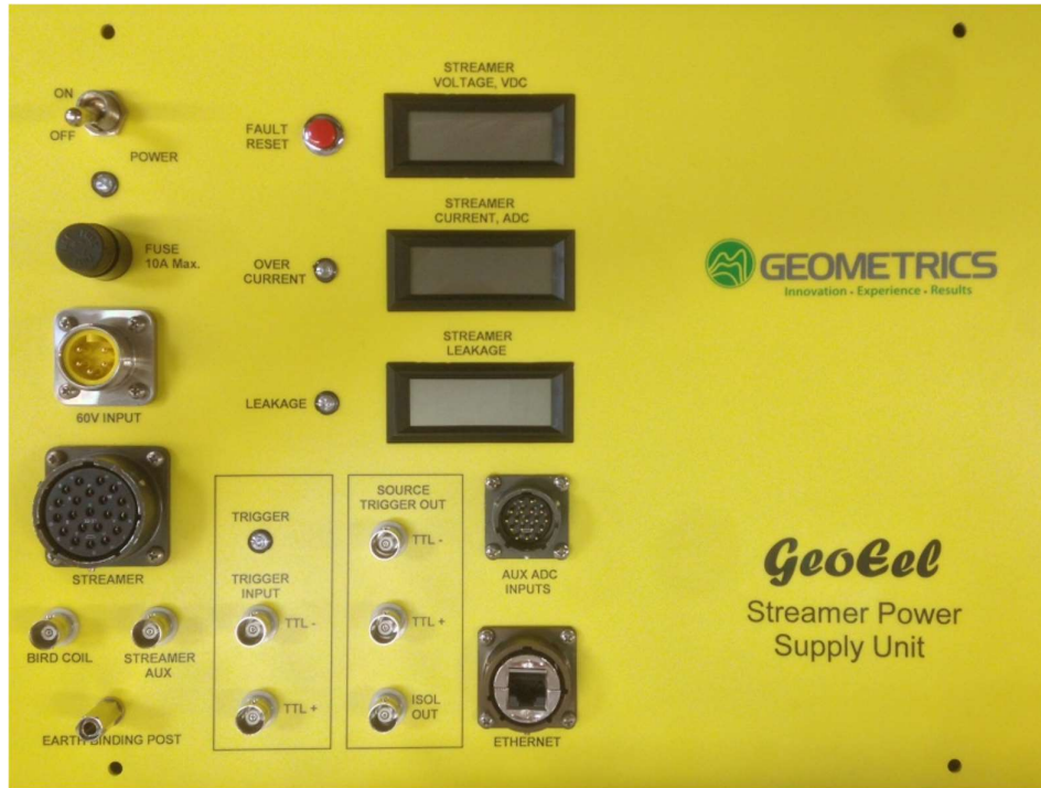
Figure 6.14: Photo showing the Portable Deck Unit front panel.
