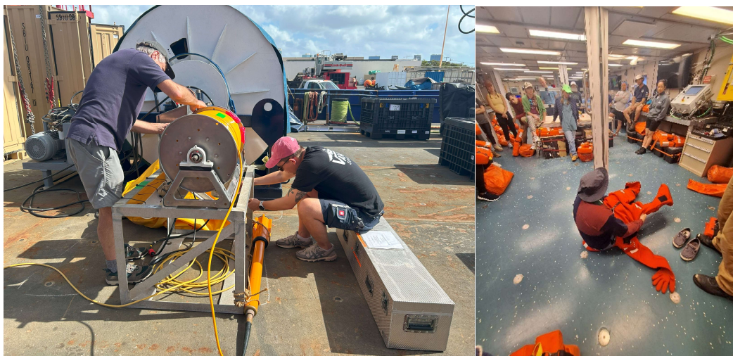
Figure A.1.1: Preparation of the SeaSpy magnetometer on the deck of RV Sikuliaq (left). Safety introduction (right). Photos: M. Tominaga & J. Preine.
