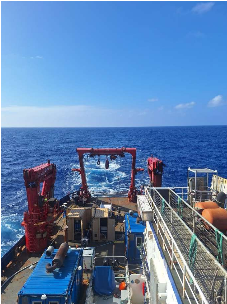
Figure A.1.42: Acquisition setup on RV Sikuliaq. The seismic streamer is towed to starboard, the airguns in the center and the magnetometer on the port side. Photo: J. Preine
