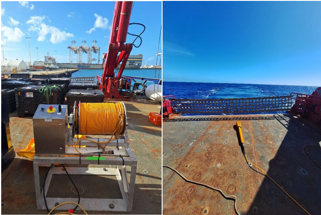
Figure 7.1: The MISO winch that aided in the deployment and retrieval of the magnetometer (left). The Marine Magnetics Seaspy2 Sensor on deck of RV Sikuliaq before deployment (right). Photos: J. Preine
