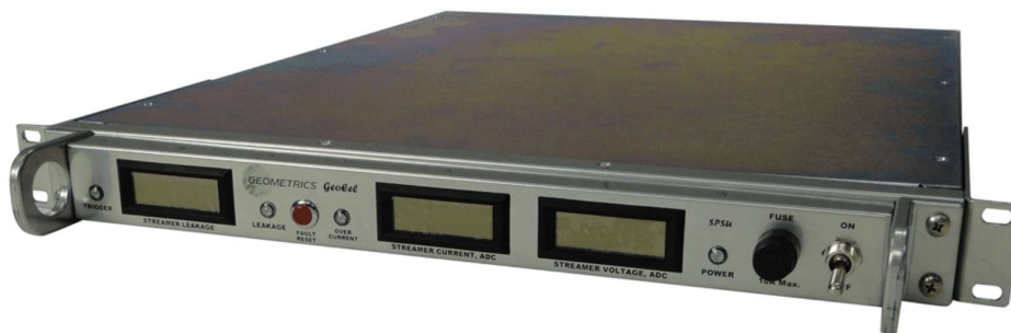
Figure 6.15: Photo showing the rack mount Deck Unit.
