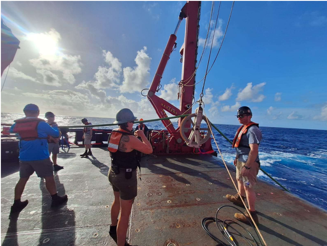
Figure A.1.34: Deployment of the seismic streamer on the deck of RV Sikuliaq. Photos: J. Preine.
