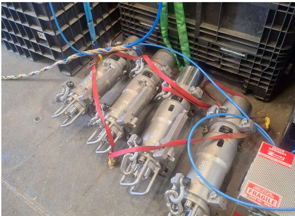
Figure A.1.25: Airguns before deployment. Photo: J. Preine.
