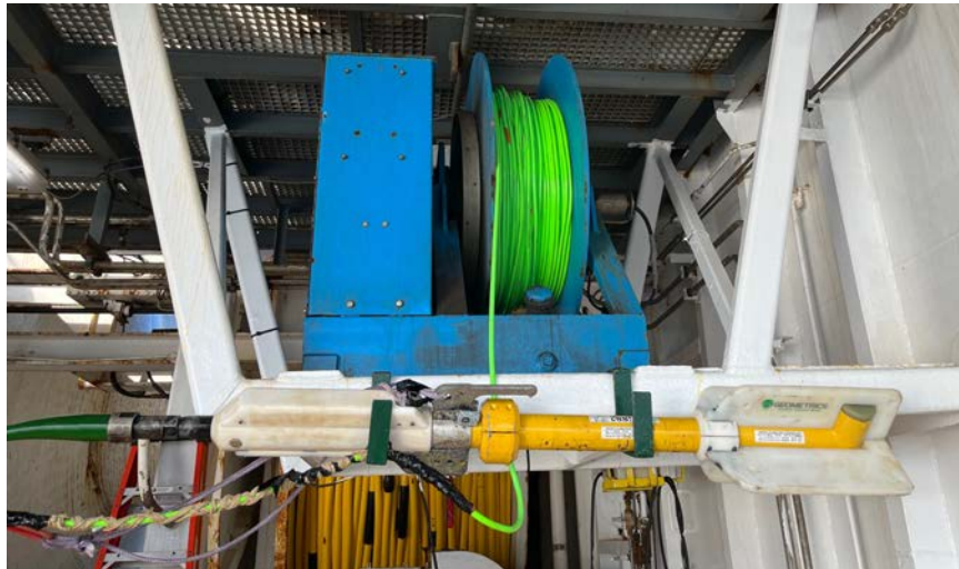
Figure 23. Photograph of GeoMetrics magnetometer and towing cable.
