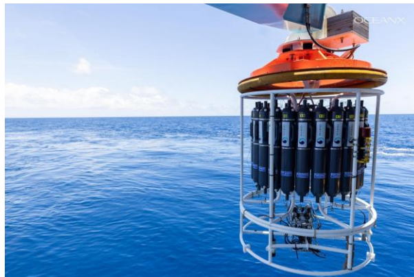
Figure 25: The CTD 'Carl' during its deployment from the starboard side of the vessel.
