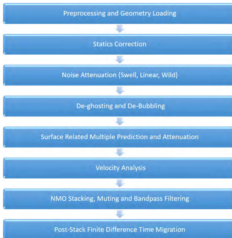
Fig 3a. Processing flow for TN-373 data visualized. The flow was constructed in GeoEast.
