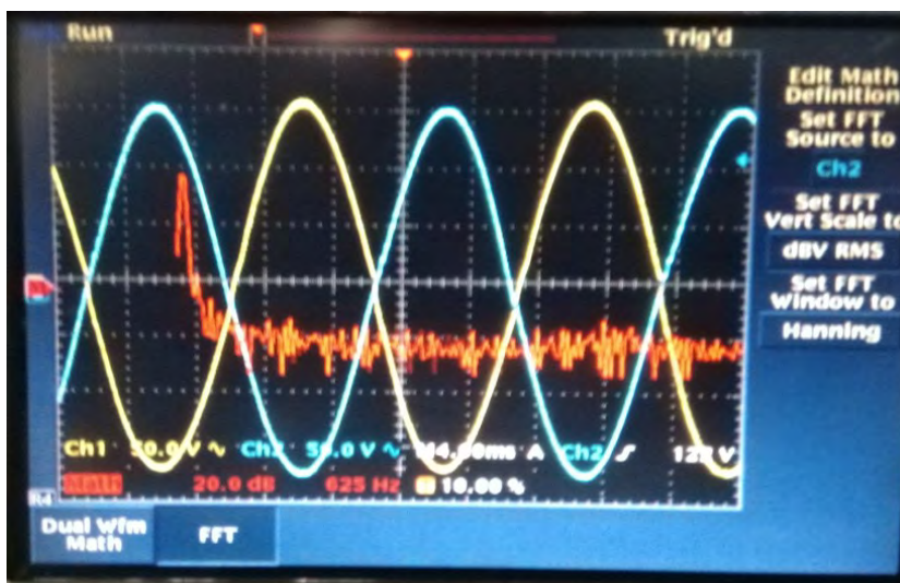
Fig5: Container UPS power output on battery, NO connection to vessel power.
