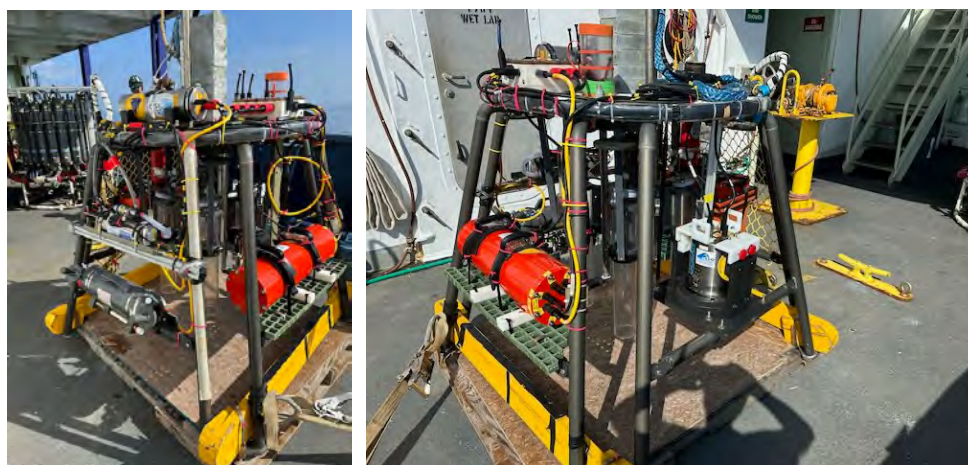
Figure A2-3. MC-400 multicorer configured with MISO imaging and data systems for AT50-09
