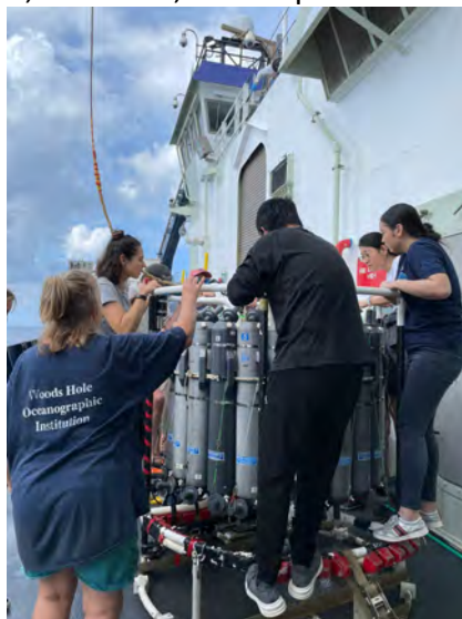
Figure 35. Preparing the CTD rosette for deployment during AT50-09.
