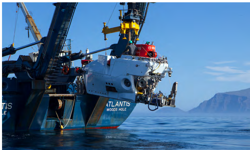
Figure A2-1b. Alvin research submarine being launched from RV Atlantis during AT50-09.
