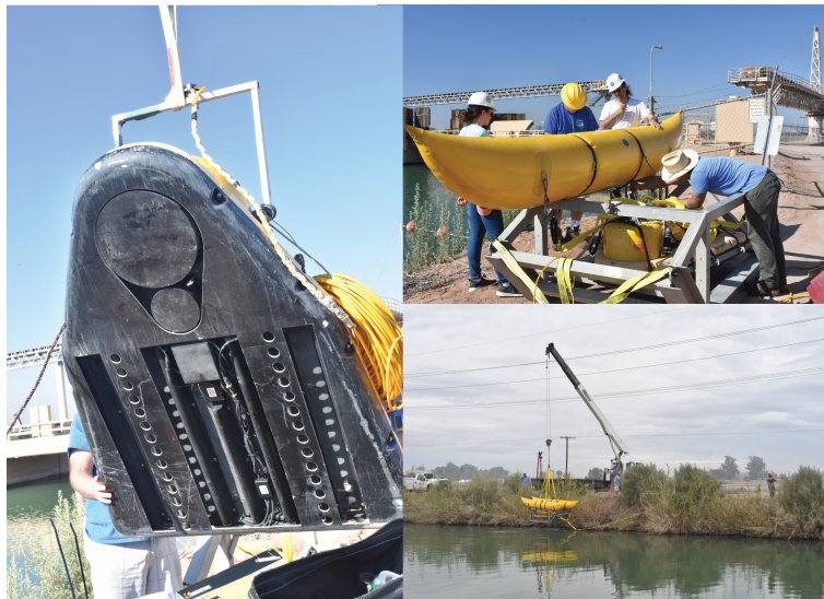
Figure 2: Images showing deployment of the CHIRP. Left: Bottom of the CHIRP, with transducers. Top right: The CHIRP in its cage, with one floating pontoon mounted. Bottom right: The CHIRP during the deployment process, with Septentrio receiver mounted on the frame.
