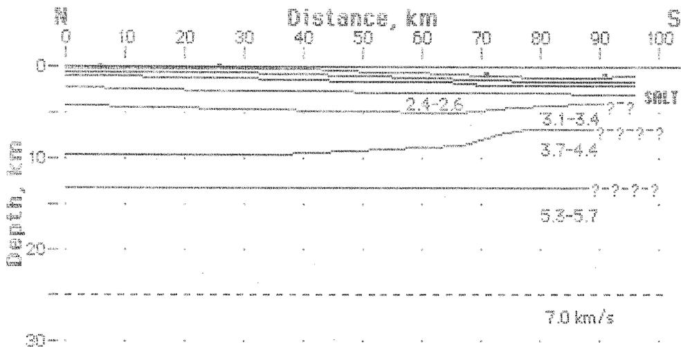
Fig. 8. Line 3 structural profile.
