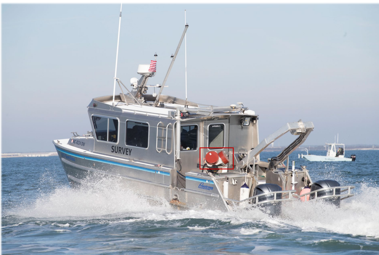
Figure 3. R/V Benthos setup with survey equipment. The red box highlights the dual-head EM2040C-D sonars.
