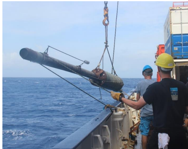
Fig. 5.10: Gravity core is lowered into the water.
