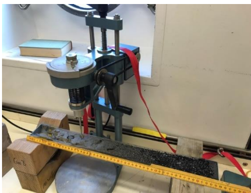
Fig. 5.21: Vane shear apparatus and GEOMAR seagoing balance.
