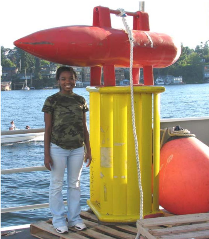
Figure 5. One of two Paravanes that connect to the cross wire and used to separate streamers. See Figures 3 and 9 for diagrammatic arrangement of the paravanes.
