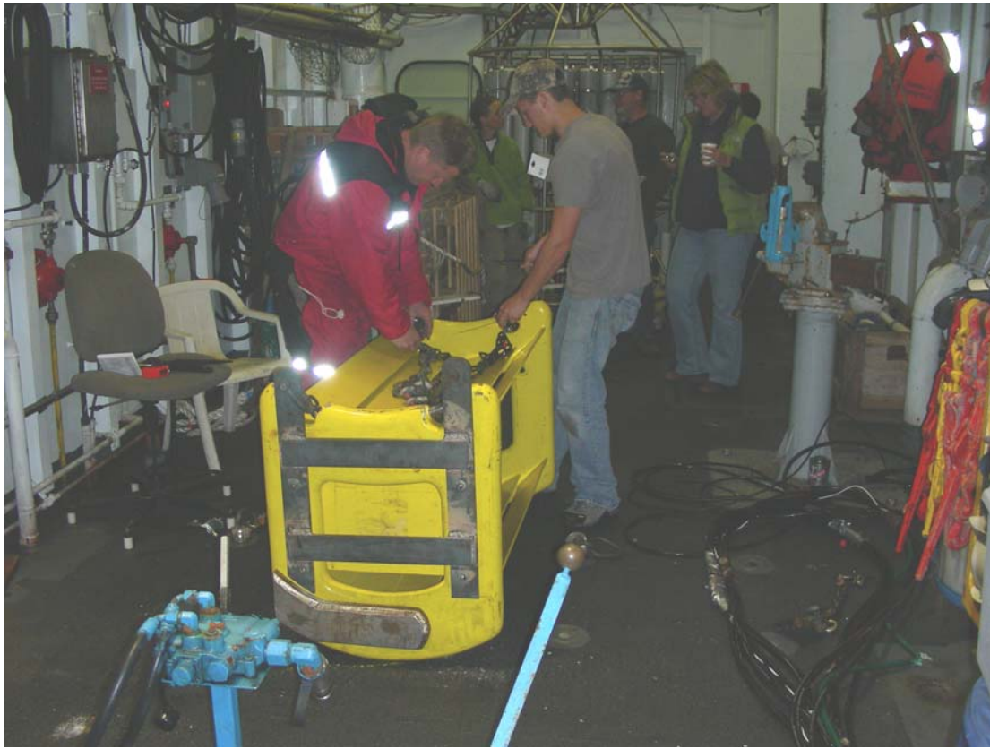
Figure 13. New steel frame that was mounted under the paravane after the towing point was damaged.
