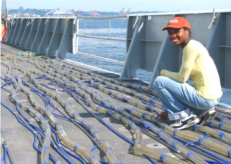
Figure 4. Streamers laid out on deck prior to deployment. Each streamer is 30 m long and is summed into a single channel.
