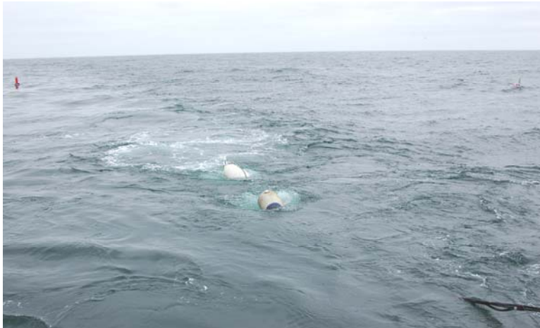
Figure 6. Seismic source towed in line from umbilicals (lower right). The port paravane can be seen in the upper right, and the center float (red boat) appears in the upper left.
