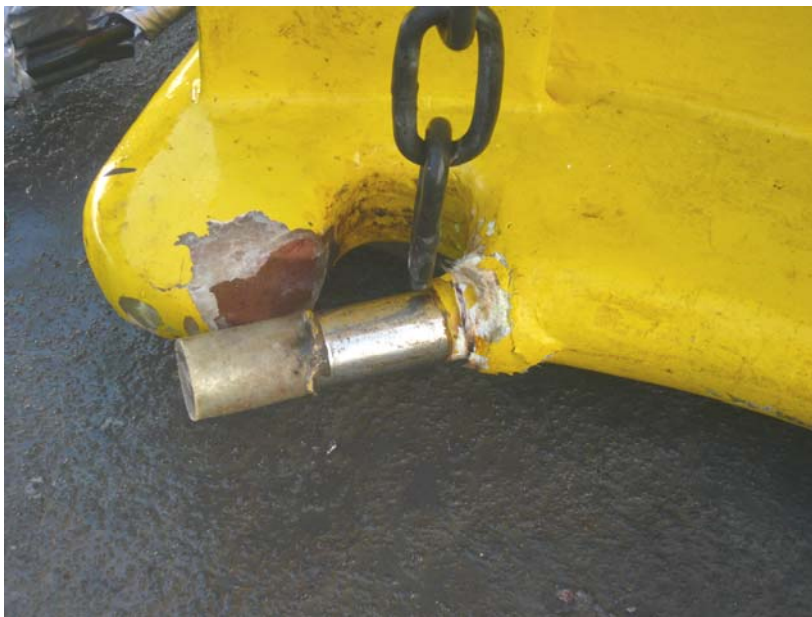
Figure 12. Damage after the lower rear chain of the port paravane was pulled out on the 7/12/08.
