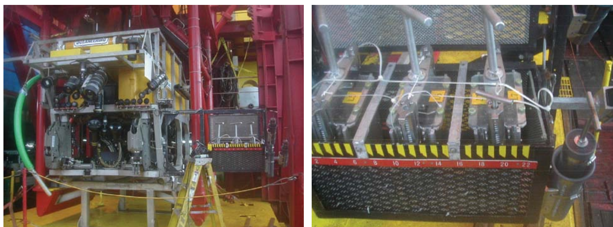
Figure 8. Left photo. ROV setup (left to right): suction sampler hose, pan-and-tilt cameras, sample basket on quadrant frame. Right photo. Sample basket containing blade cores; pushcores and quivers were mounted to the right of basket.
