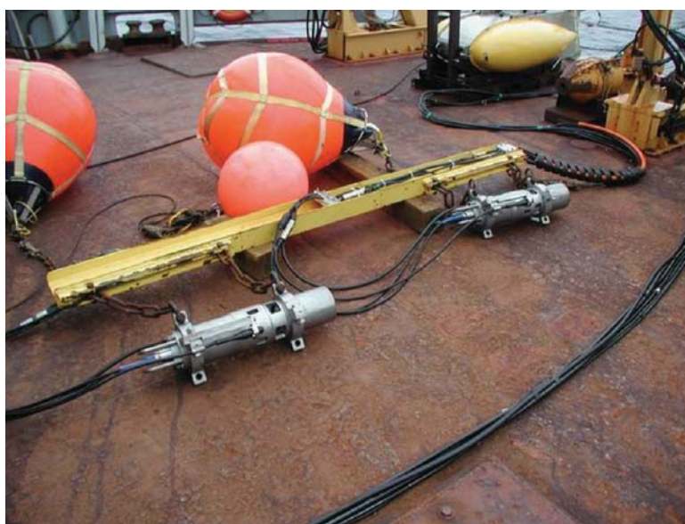
Figure 2. The two air gun array on the fantail of M/V The Performer
