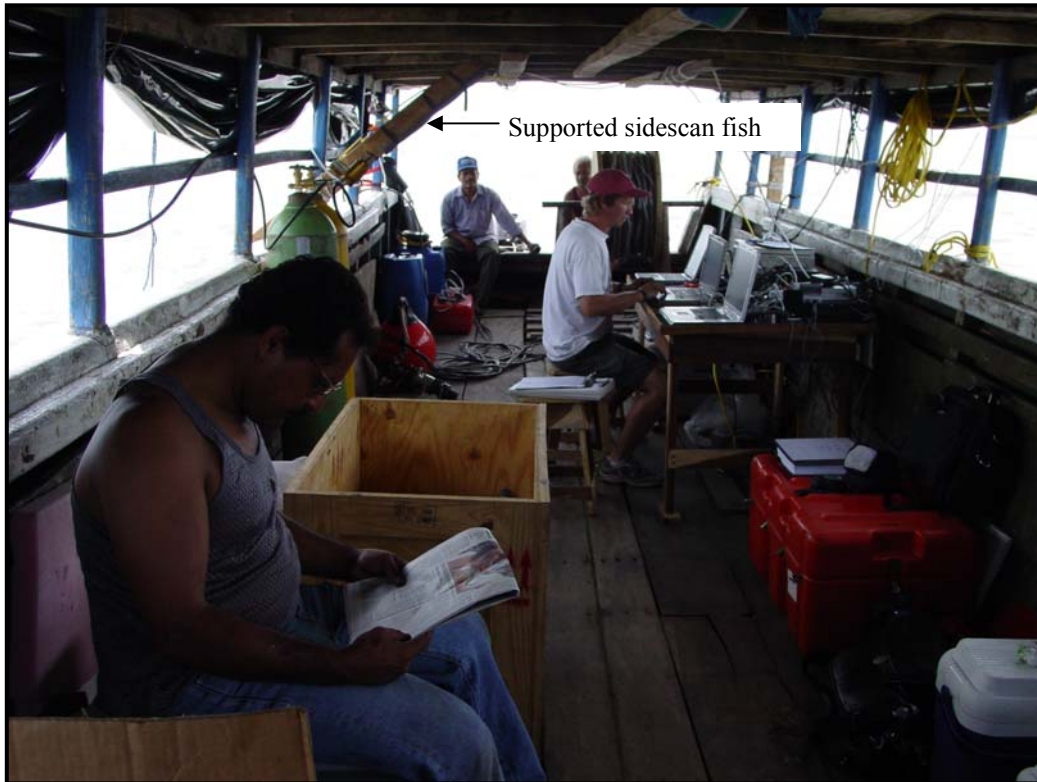
Figure 25. Steffen Saustrup is maintaining the laptops aboard the Morrito No. 2 during the Lake Managua survey. The board wedged against the upper deck in the top left of the picture extends out into the water, supported the sidescan sonar “fish”. The “fish” hung by a carabineer from the plank at ~1 m water depth.
