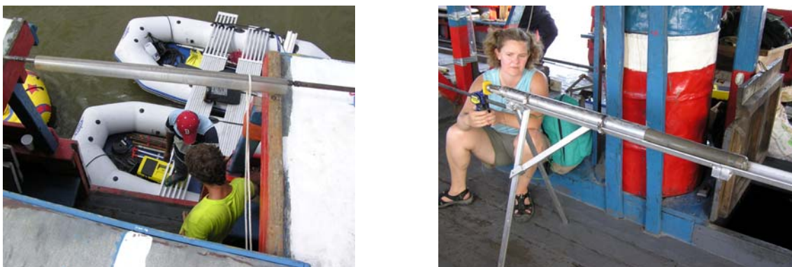
Figure 31. A) Preparation of coring raft used for the retrieval of piston cores. B) Extrusion procedure of piston cores (photos: Robert Dull)
