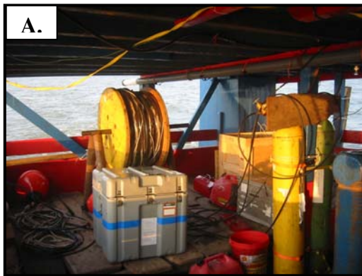
Figure 21. A) The streamer was set up in the middle near the stern of the Mozorola . Two high pressure holding tanks fed the air gun and were fastened to a center column of the ship. The air gun was positioned on the starboard side of the Mozorola , secured to a retractable plank. B) Aboard the Morrito No. 2 , everything was wired to a central computing system positioned on the port side of the vessel.
