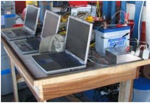
Fig. 13. Laptop/Geode/Shotbox set-up in the field: Nicaragua, 2006.
