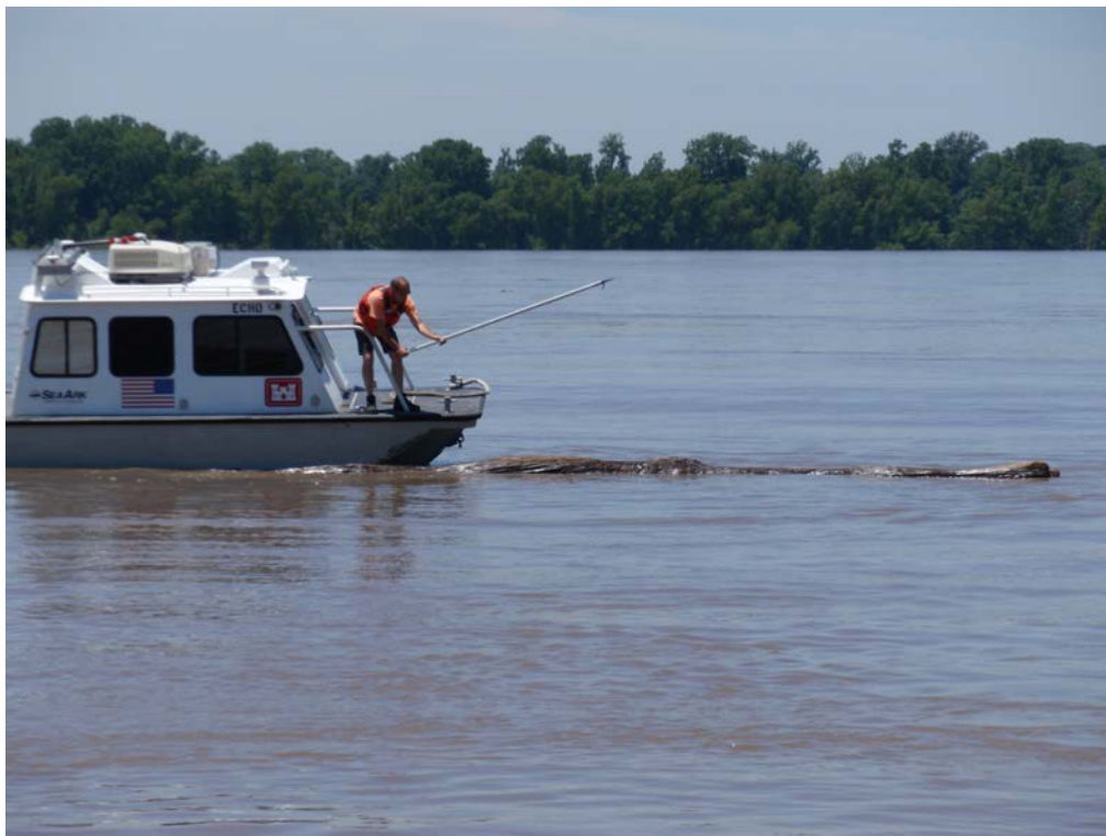
Figure 5. Chaser boat clearing an incoming log away from the path of the streamer and airgun.
