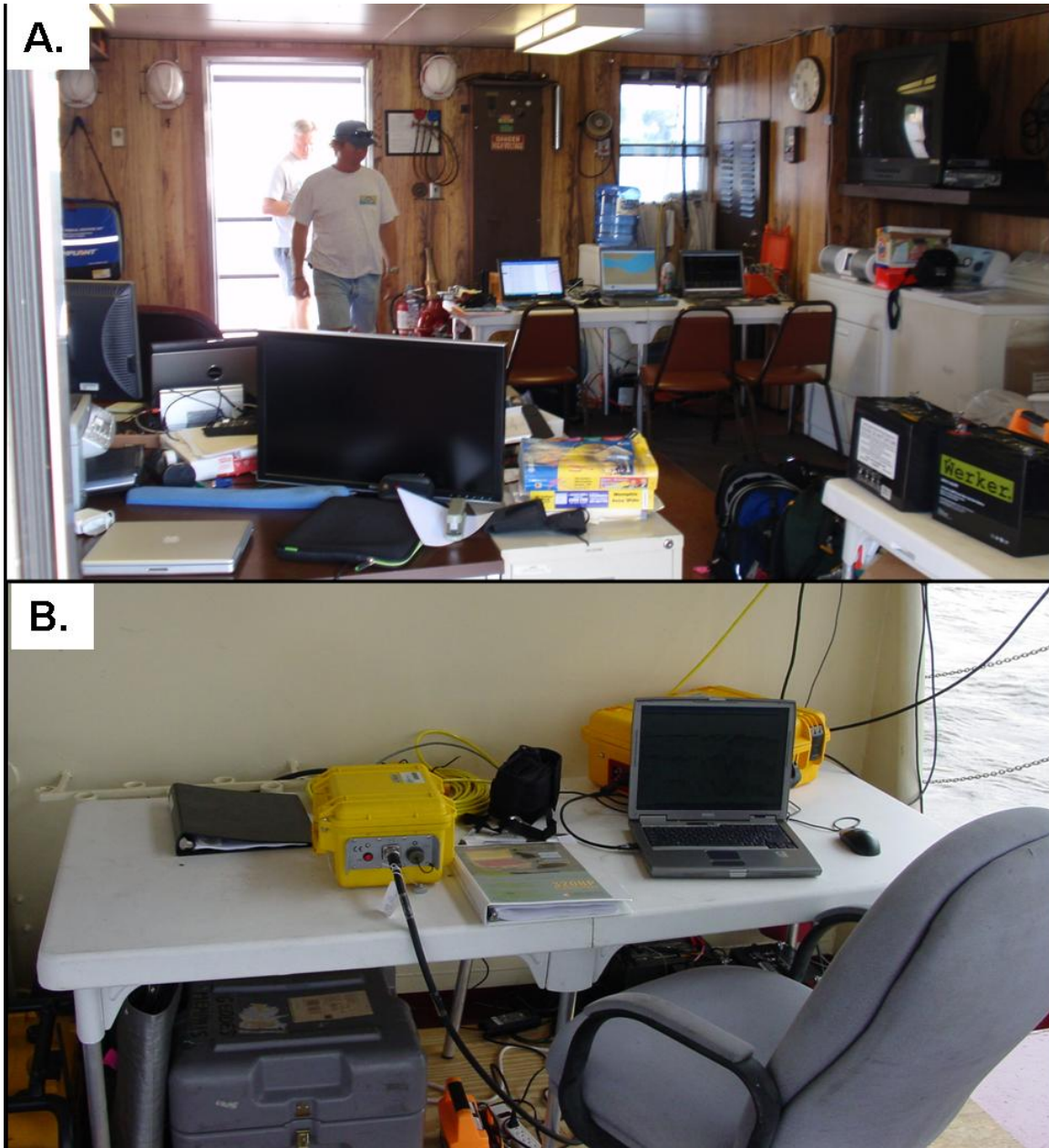
Figure 8. A.) Inside seismic lab and (B.) Echosounder outside lab setups.
