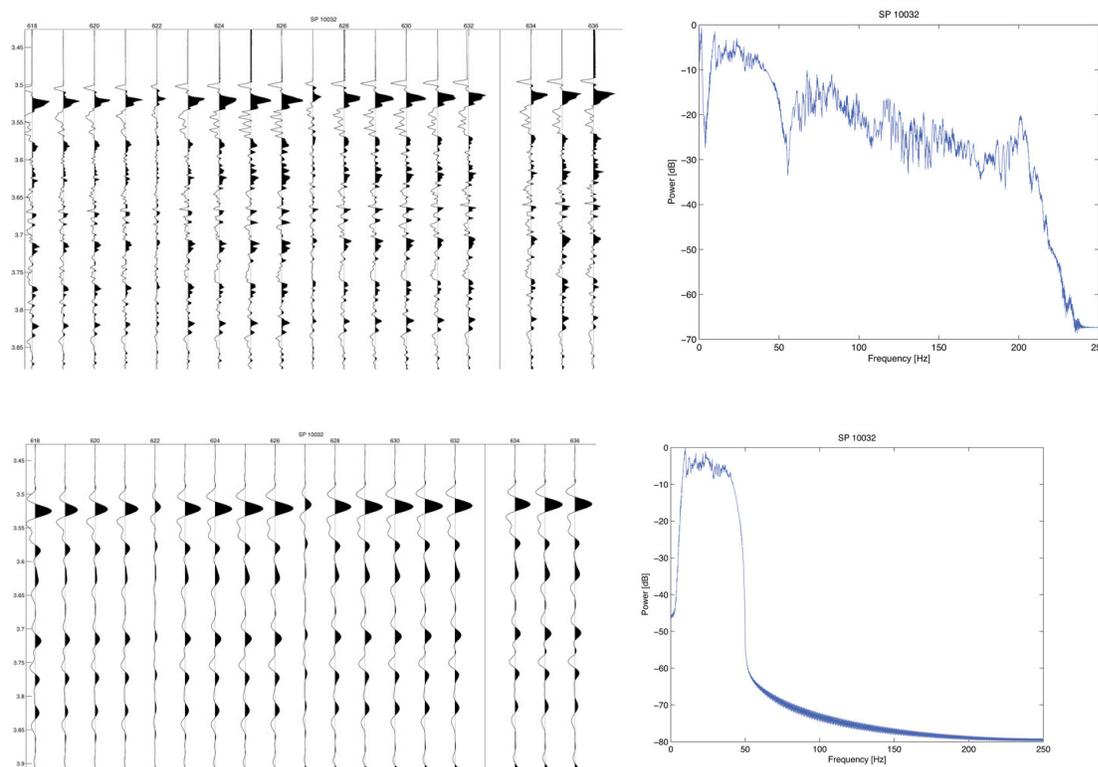
*Figure 27. (Top left) Seafloor reflection on inner traces of shot gather from SP 10032, seaward of the trench on Line 5, when guns were at 15 m depth. (Top right) Frequency spectrum of shot gather, showing clear ghost notch at 50 Hz, as expected. (Bottom left) Same traces, filtered from 10-40 Hz. (Bottom right) Frequency spectrum after filtering.*
