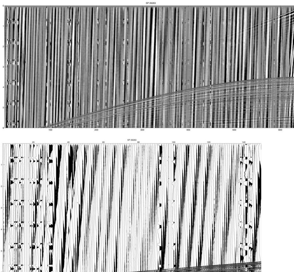
*Figure 30. (Top) Raw, unfiltered data from Line 4, SP 26263, showing noise bursts. The noise is apparent as bright “glitches” that tend to occur at the same time on numerous traces. (Bottom) Zoom of outer portion of streamer, showing waveform of noise in wiggle-trace format.*
