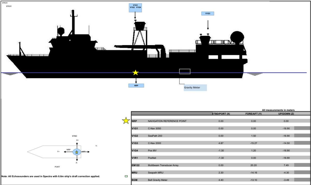
Figure 16. Antenna locations on R/V Langseth during MGL1212.
