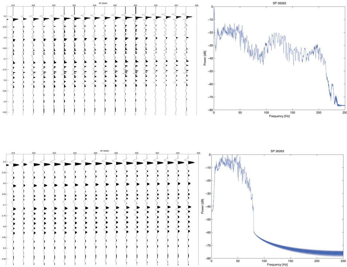
*Figure 28. (Top left) Seafloor reflection on inner traces of shot gather from SP 26263, seaward of the trench on Line 4, when guns were at 9 m depth. (Top right) Frequency spectrum of shot gather, showing ghost notch at 83 Hz, as expected. (Bottom left) Same traces, filtered from 10-70 Hz. (Bottom right) Frequency spectrum after filtering.*
