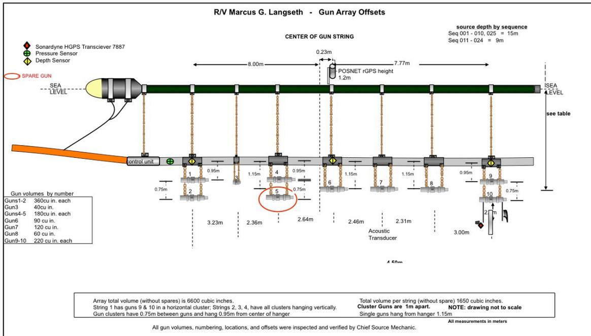
Figure 14 (above). Gun array offsets during MGL1212.
