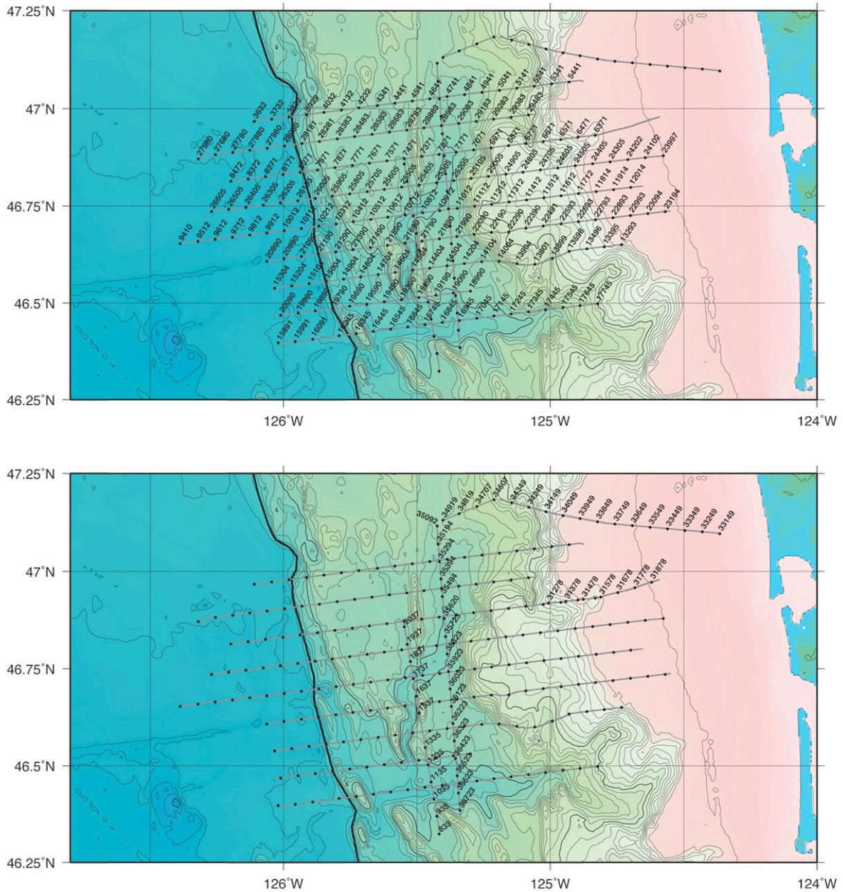
Figure 4. Map of actual track lines, along with indications of gun array status during shooting. This map provides an “at-a-glance” look at survey completion, by comparing thick black lines (full array shooting) to green lines (original plan).
