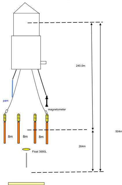
Figure 15 (left). Tow configuration of the gun strings during MGL1212.
