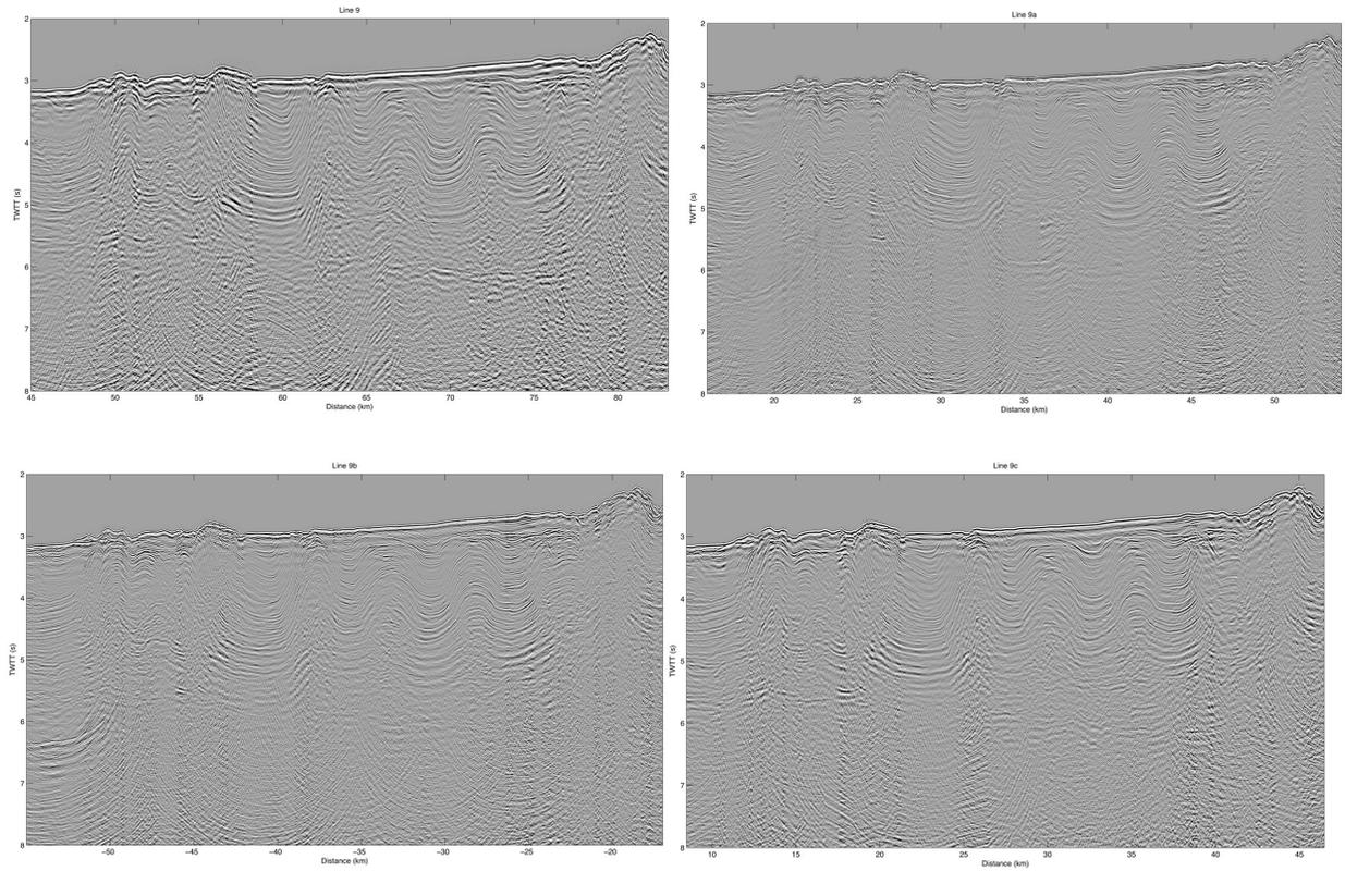
*Figure 29. Comparison of same area shot with four different source configurations. (Top left) Line 9, full source array at 15 m depth. (Top right) Line 9a, full source array at 9 m depth. (Bottom left) Line 9c, half source array at 15 m depth. (Bottom right) Line 9d, half source array at 15 m depth.*
