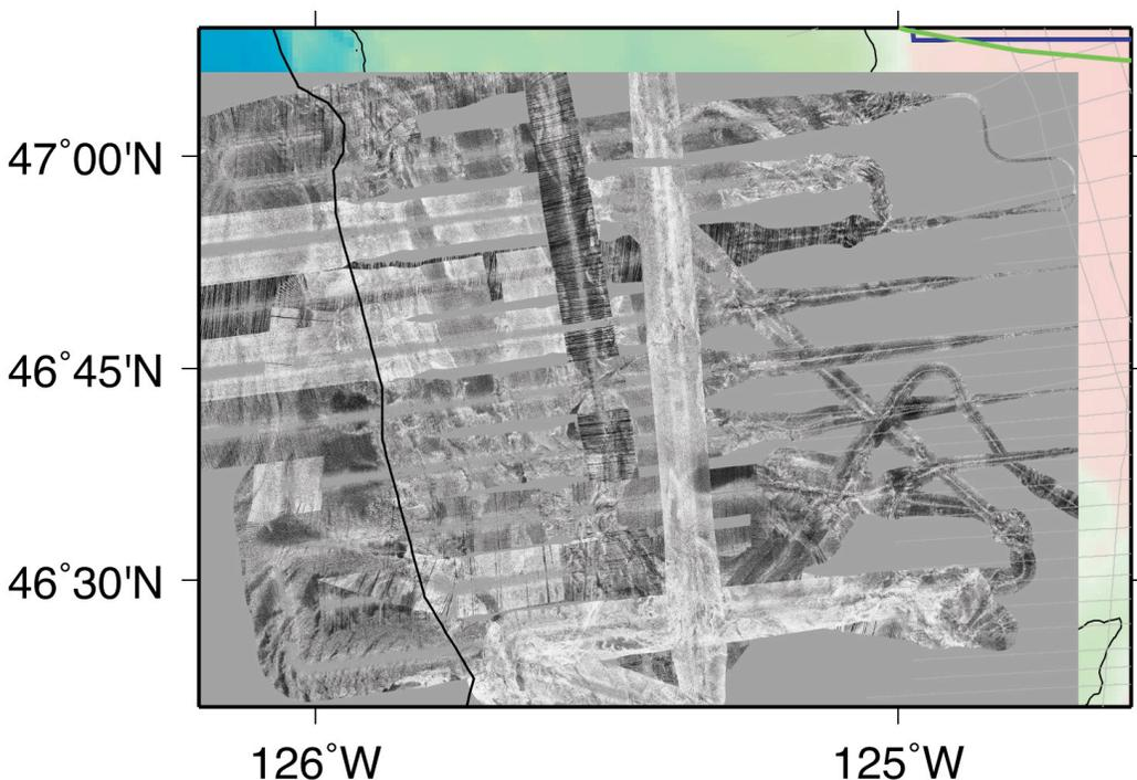
Figure 36. Image of all sidescan data collected during MGL1212.
