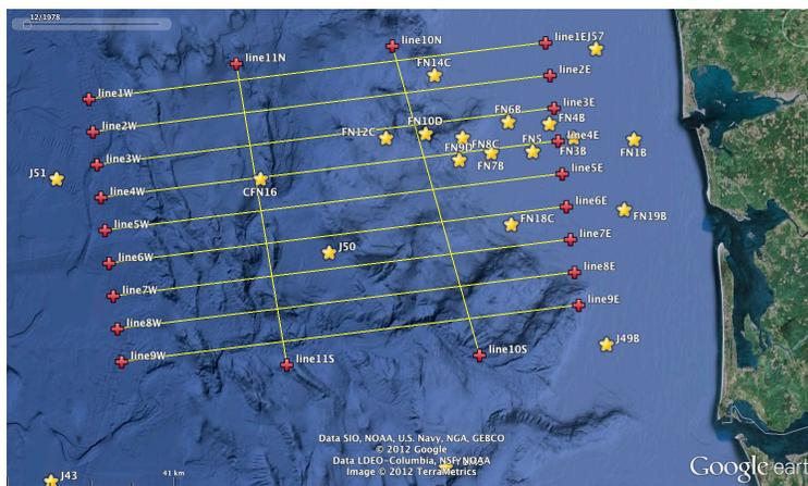
Figure 3. Map of planned track lines, plotted with positions of Cascadia Array ocean-bottom seismometers.
