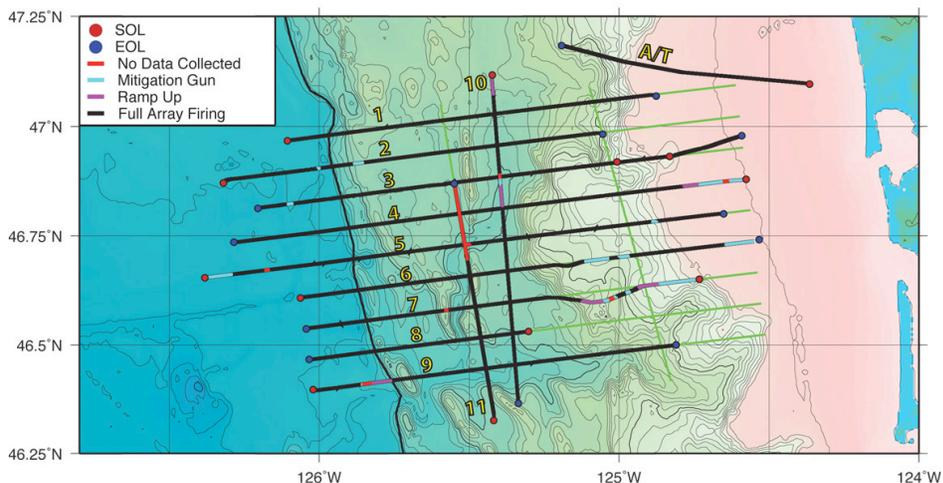
Figure 2. Map of actual track lines, along with indications of gun array status during shooting. This map provides an “at-a-glance” look at survey completion, by comparing thick black lines (full array shooting) to green lines (original plan).
