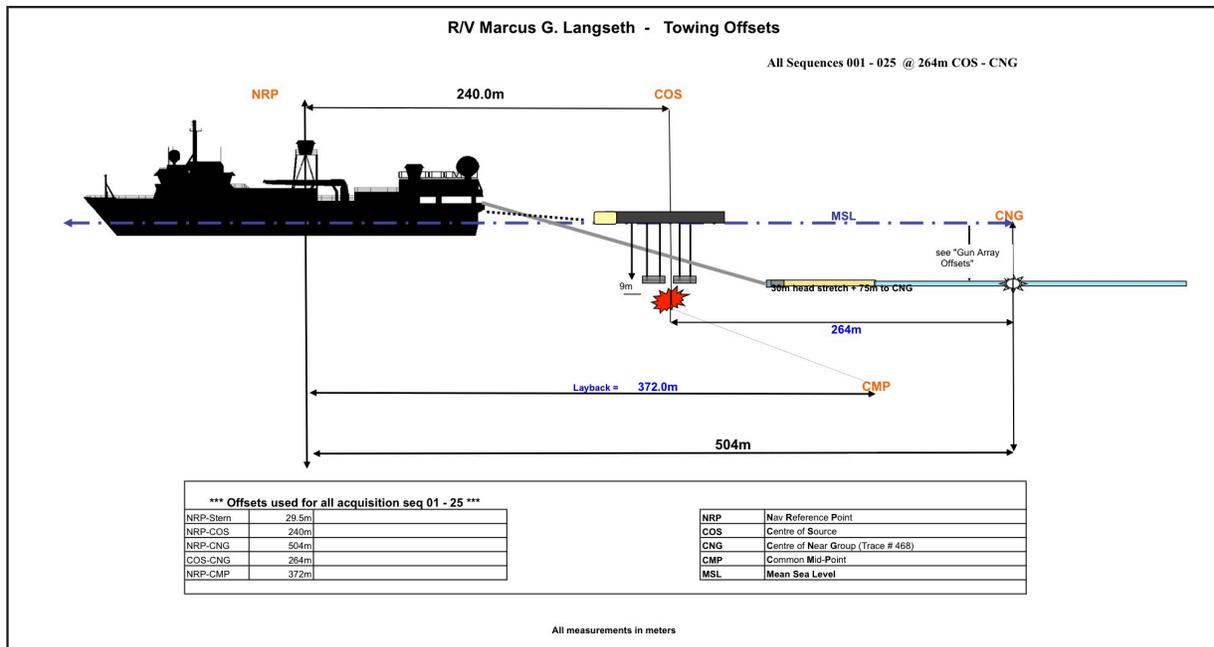
Figure 13. Setback diagram of MGL1212. Source-to-near-channel offset was 264 m.
