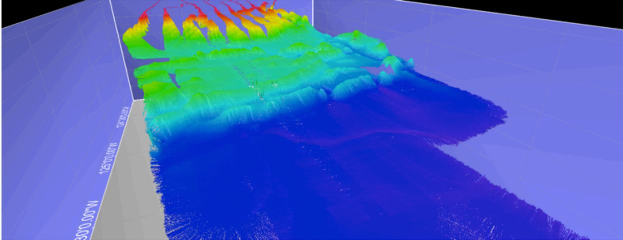
Figure 32: Exported 3D visualization of collected multibeam
