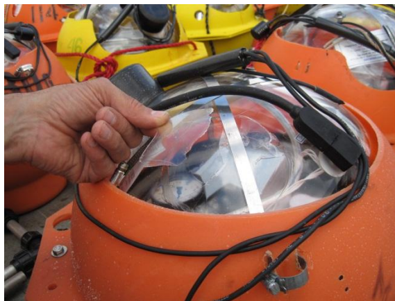
Figure 6.24. Glass shards peeling off recovered OBS. This OBS may have hit the hull during an earlier recovery in rough weather, causing stress to the sphere.
