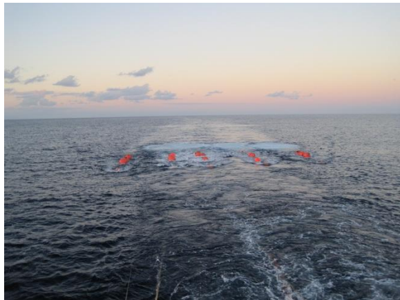
Figure 6.6. Shooting three of five air gun strings towed by the M/V Iron Cat .
