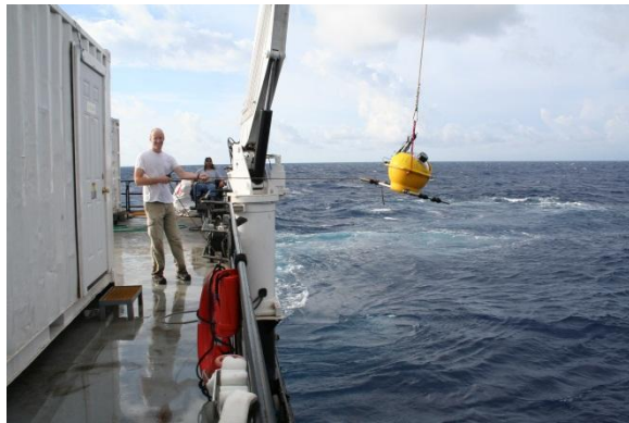
Figure 6.10. Lifting an OBS from lower to upper deck after recovery.
