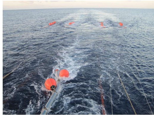
Figure 6.22. Deploying an air gun string.
