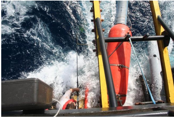
Figure 6.21. Air gun string recovery in rough weather.
