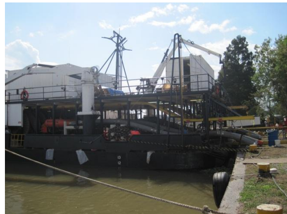
Figure 6.26. Stern of the M/V Iron Cat . Air gun arrays are visible on the lower deck; containers on the top deck provided storage space, the OBS lab, and living quarters.
