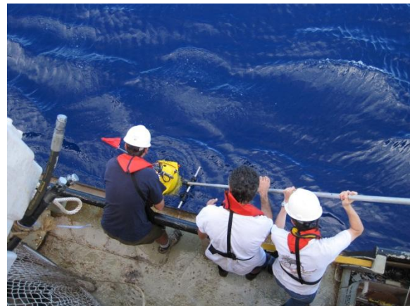
Figure 6.4. Recovery of an OBS from the lower deck using a boat hook. The crane is then used to lift the OBS to the upper deck.
