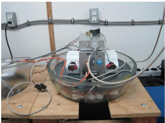
Figure 6.23. Open OBS sphere. Visible are batteries, the Sedis-V computer, and the acoustic release unit.
