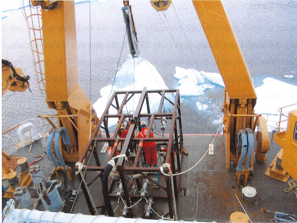
Figure 4. View of seismic source frame from above. Frame towed by main trawl wire.
