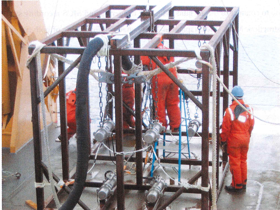
Figure 2. Airgun frame from forward end showing cement pipe with airlines and firing lines. All four GI guns are installed. Central tow point at center-top of frame.
