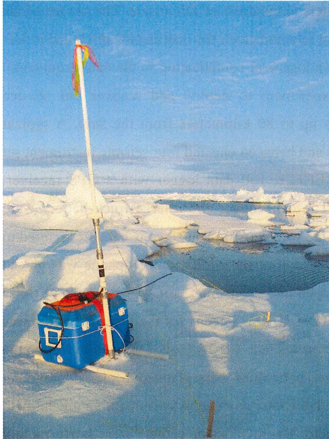
Figure 1. Initial deployment method using guy-lines to secure antenna mast. It was determined that guy-lines were not useful since tentpegs melted out.
