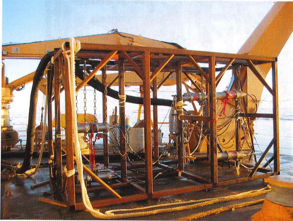
Figure 1. Airgun frame with initial installation of some airguns. GI guns are to the left, Bolt guns are to the right. Lower forward GI gun not yet installed.
