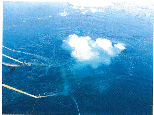
Figure 6. Seismic source frame deployed. Tag lines can be seen in photo above and photo on the right. Typical ice conditions on Chukchi and Mendeleev ridge profiles. Ice conditions on Northwind Ridge were much worse.
