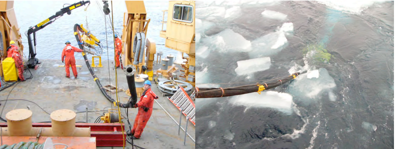
Figure 13 – Deploying the guns and streamer.
