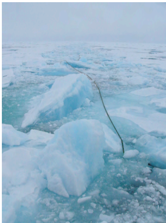
Figure 16 – The streamer was left on the ice twice during the cruise for a loss of 5 streamer sections. This would happen when ice got under the airguns, lifting them out of the water. The streamer, threaded through the wing carrying the guns, would follow, dragged across the ice. If ice crowded into the wake, it could pinch and strand the streamer on the ice surface.
