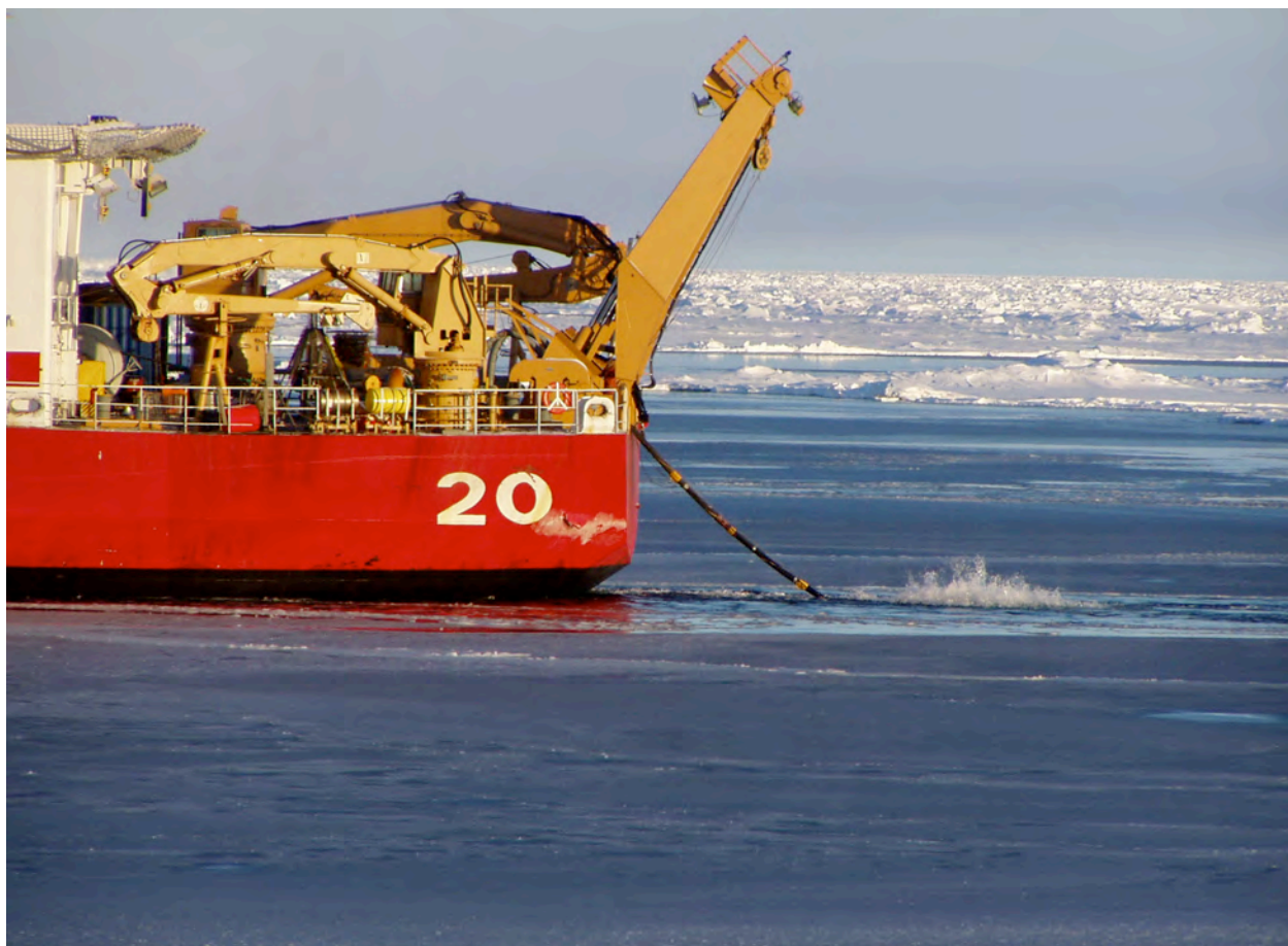
Figure 15 – Towing in an open lead. These are excellent conditions for MCS data acquisition.
