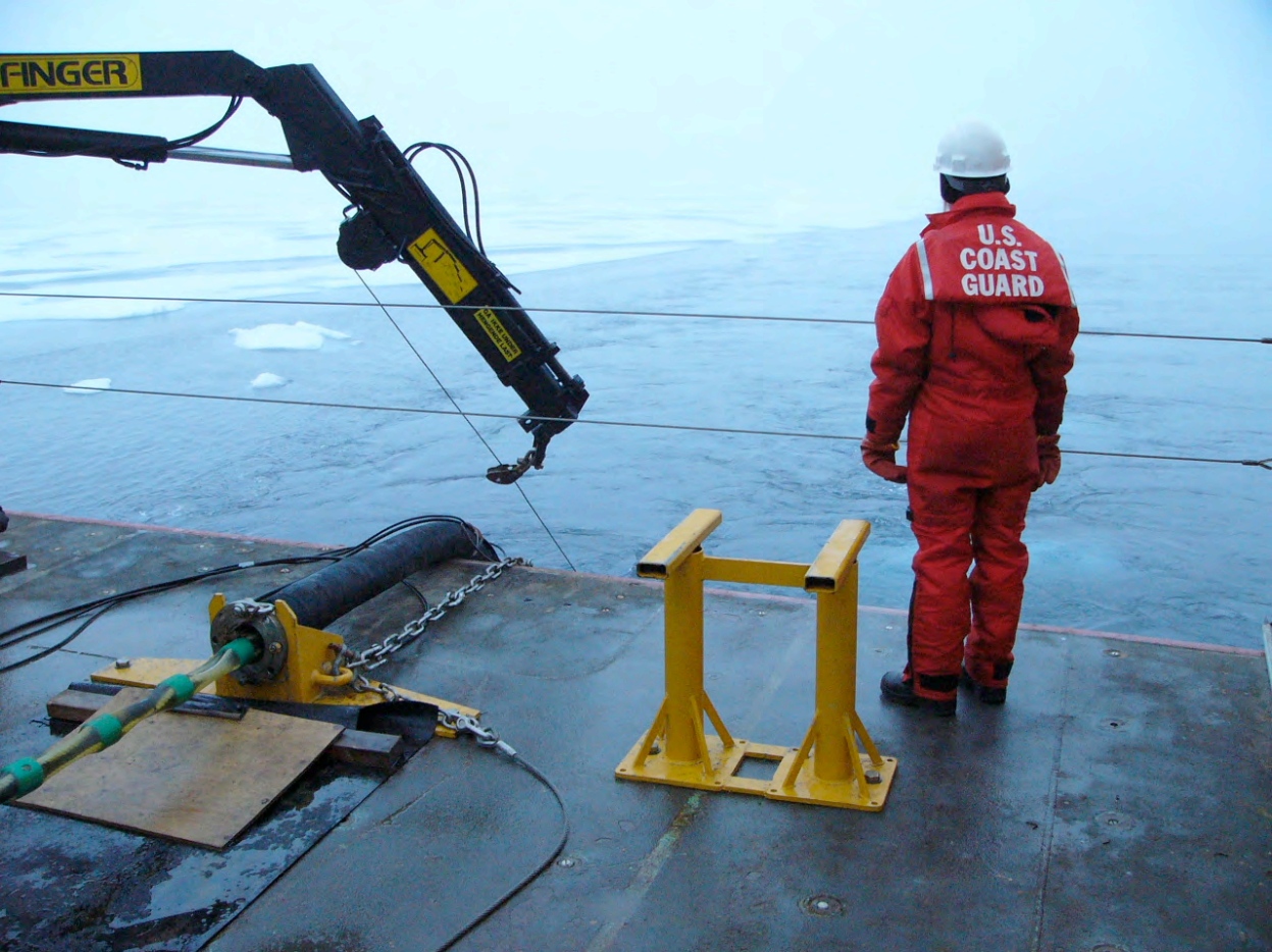
Figure 14 – While the MCS gear was deployed, a watch was stationed on the fantail to make sure towing did not result in fouling of the gear. This watch was in direct communication with the bridge, which was instructed to stop upon their request. This did not always work well owing to occasional poor radio reception and misunderstandings.
