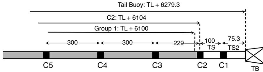
*R/V Ewing streamer geometry for Lau experiment*
