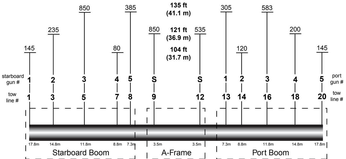
*R/V Ewing gun array showing gun numbers and chamber sizes. The two guns on the A-frame, marked S, were spare guns used to replace the 850 cu. in. & 583 cu. in. guns when they went down*
