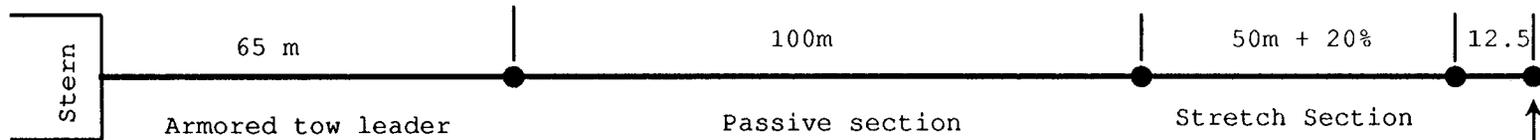
CABLE = 160 CHANNEL- 40 ACTIVE SECTIONS- 4264 METERS TOTAL LENGTH
