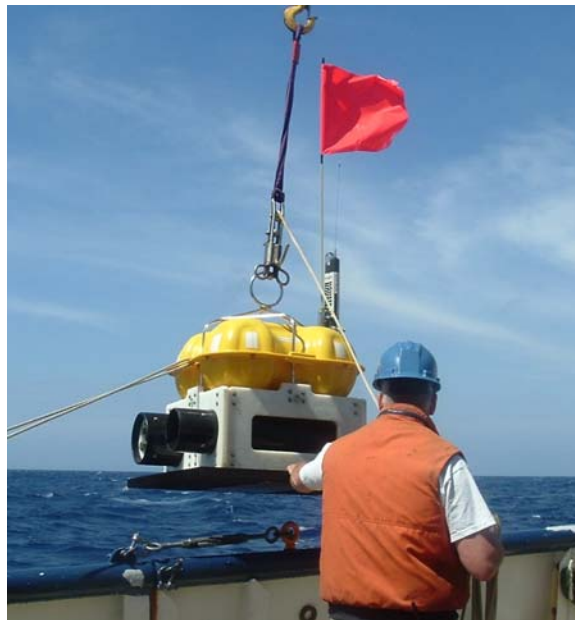
Figure 4. Deployment of Scripps LC2000 OBS.
