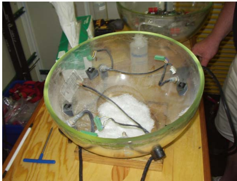
Figure 5. Glass powder within instrument ball for D57.
