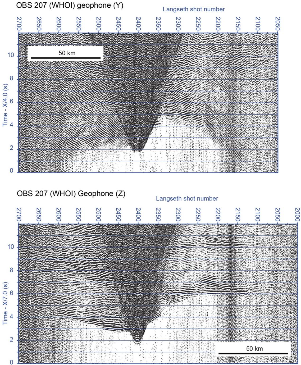
**Figure 14b.** Shot line OBS002 record sections of OBS 207. This was an instrument from the WHOI OBSIP group. Top: Horizontal channel (3). Bottom: Vertical channel.
