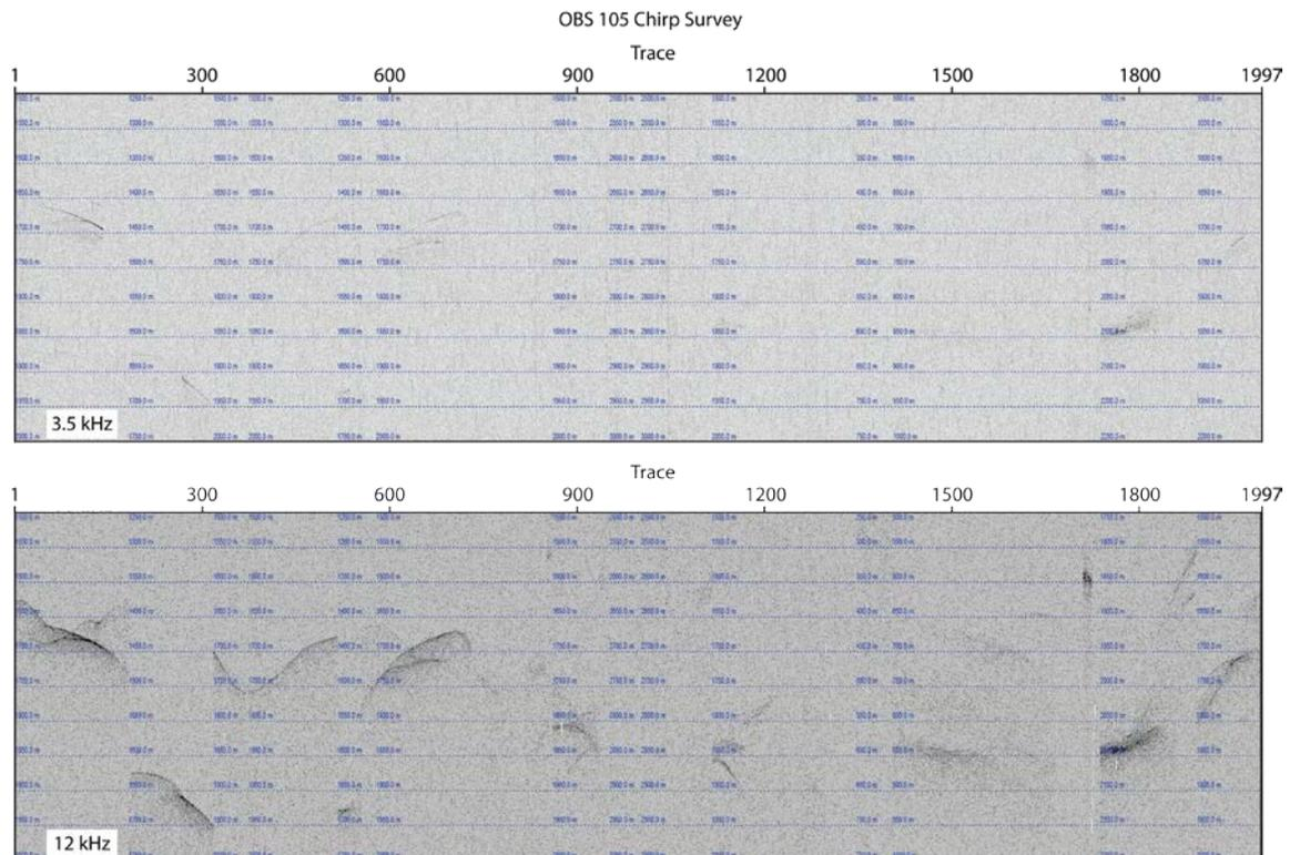
**Figure 9.** Raw 3.5kHz (top) and 12kHz chirp survey for OBS 105. Trackmap for survey is located in Figure 8. Depth scale varies along the profile (blue lines) based on changes in water depth and dynamic chirp scale adjustments.
