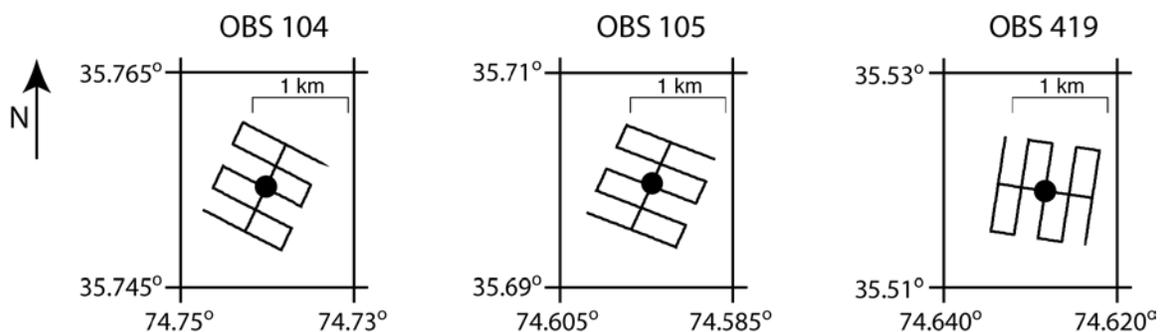
**Figure 5.** Planned survey grids over proposed sites for OBS 104, OBS 105, and OBS 419. Proposed OBS locations (solid black dots) are the center of the surveys which extend 500 m away from the sites.
