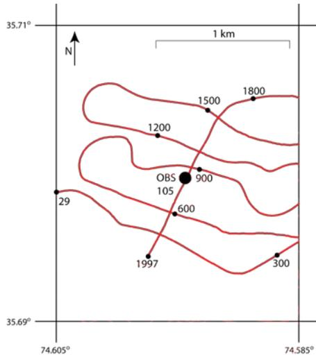
**Figure 8.** Track map for seafloor environmental survey over proposed location for OBS 105 (red line). Proposed OBS site is large black dot. Small, numbered dots are chirp trace numbers.
