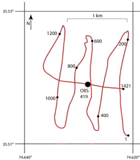
**Figure 10.** Track map for seafloor environmental survey over proposed location for OBS 419 (red line). Proposed OBS site is large black dot. Small, numbered dots are chirp trace numbers.
