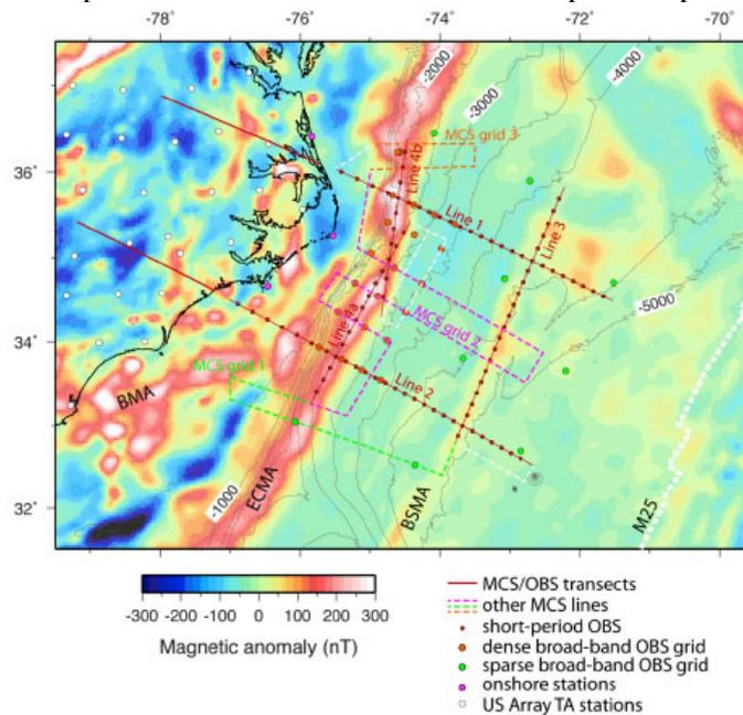
**Figure 2.** Instrument layout and transects of the ENAM Community Seismic Experiment with some modifications adopted in December 2013. Some additional changes were made in the MCS coverage during data acquisition in September and October 2014.
