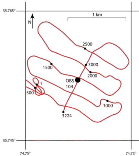
**Figure 6.** Track map for seafloor environmental survey over proposed location for OBS 104 (red line). Proposed OBS site is large black dot. Small, numbered dots are chirp trace numbers.
