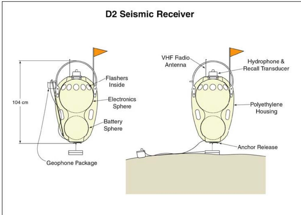
**Figure 4.** Schematic layout of the WHOI D2 OBS.
