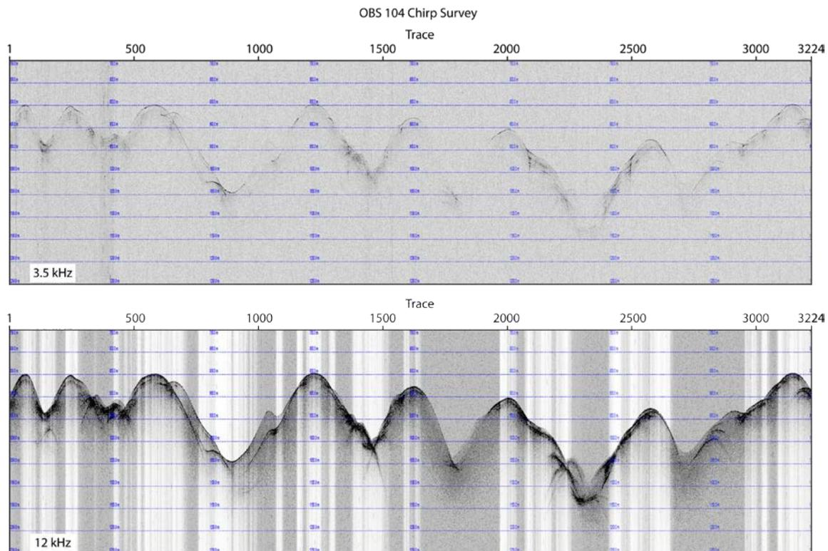
**Figure 7.** Raw 3.5kHz (top) and 12kHz chirp survey for OBS 104. Track map for survey is located in Figure 6. Depth scale is constant from 750-1250 m water depth across the profiles.
