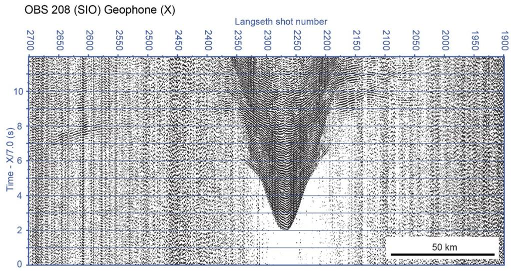
**Figure 15a.** Shot line OBS002 record sections of OBS 208. This was an instrument from the SIO OBSIP group. Top: Hydrophone channel. Bottom: Horizontal channel (X).
