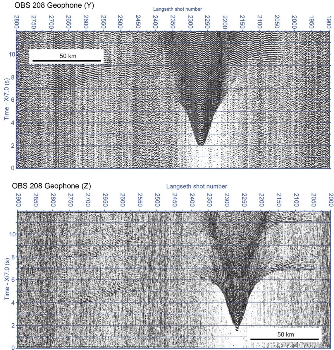
**Figure 15b.** Shot line OBS002 record sections of OBS 208. This was an instrument from the SIO OBSIP group. Top: Horizontal channel (Y). Bottom: Vertical geophone channel.
