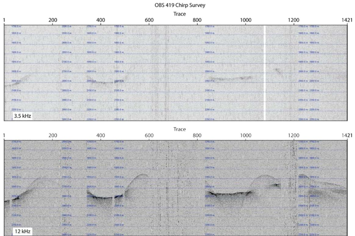
**Figure 11.** Raw 3.5kHz (top) and 12kHz chirp survey for OBS 419. Trackmap for survey is located in Figure 10. Depth scale varies along the profile (blue lines) based on changes in water depth and dynamic chirp scale adjustments.
