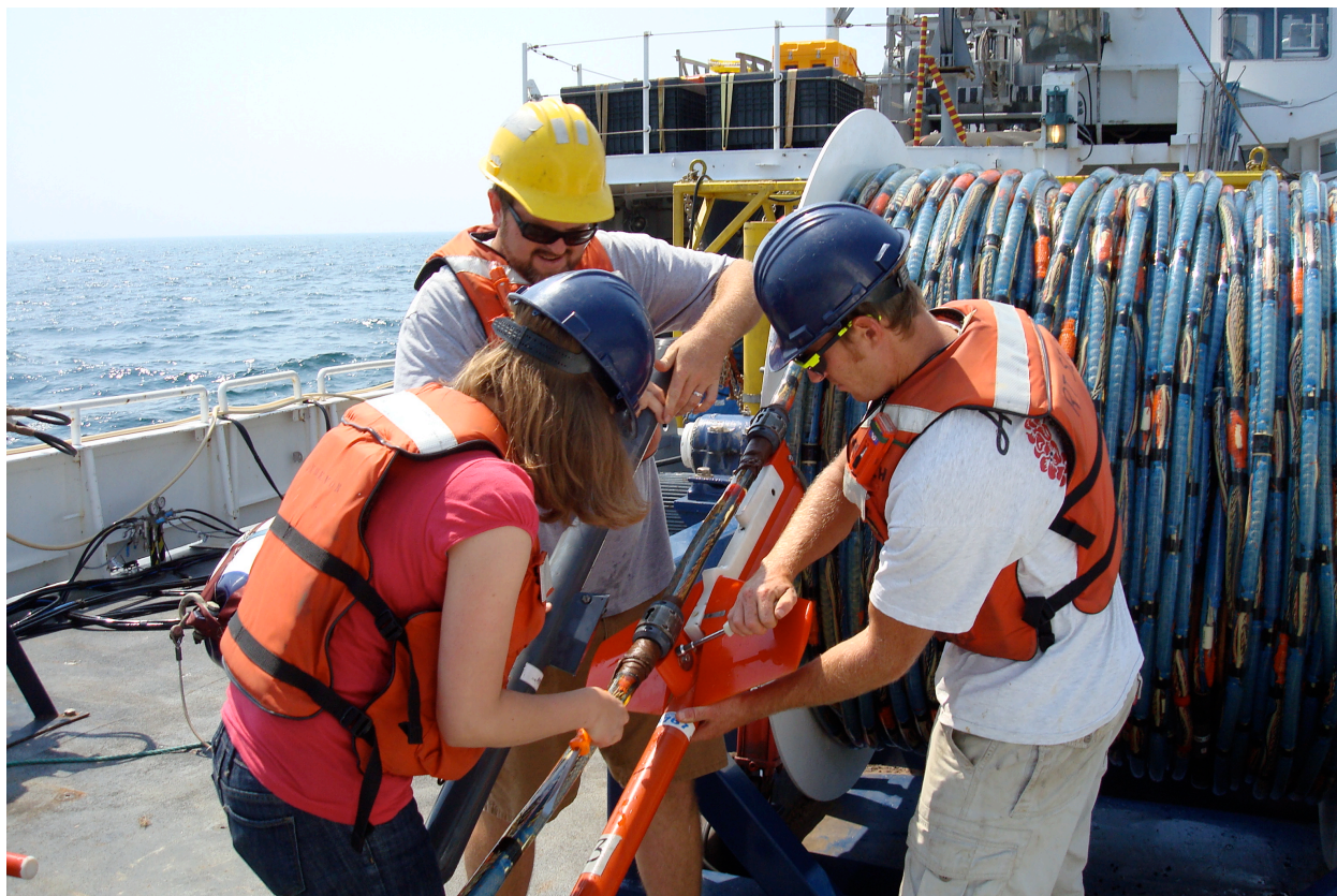
Figure 5. Connecting one of the depth-control birds on the high-resolution, multi-channel streamer.
