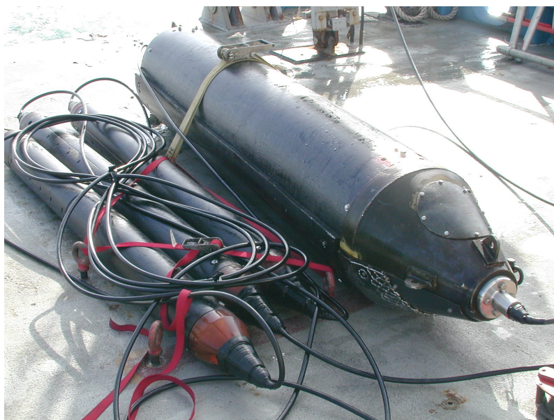
Figure 7. A photograph of the WHOI towed EM system on deck. The system consists of a transmitter (large cylinder at right) connected to the ship by a 0.680 conducting cable. Three receivers (smaller cylinders) to behind the transmitter at separations of 4m, 13m and 40m and provide information to depths of about 20m subsurface.
