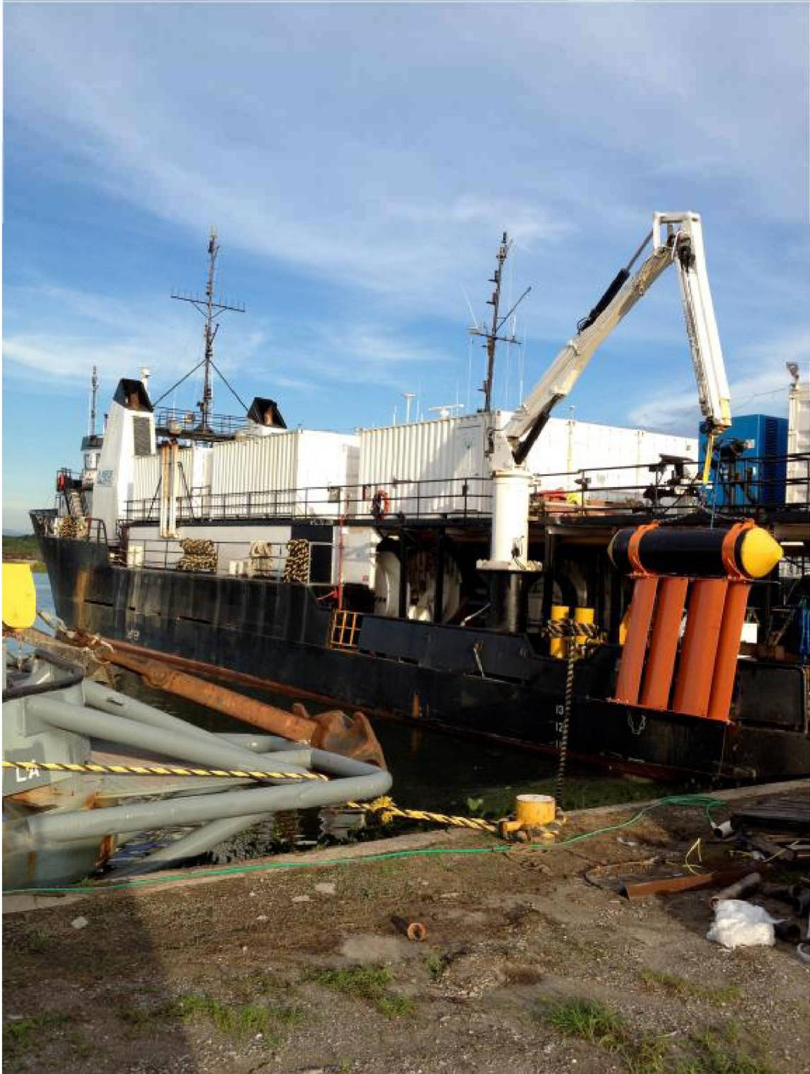
Figure 8.6: Photo showing the R/V Iron Cat at a dock in the port of Amelia, LA. Note the bright orange-colored paravanes and black and their yellow floats strapped to the side of the ship.
