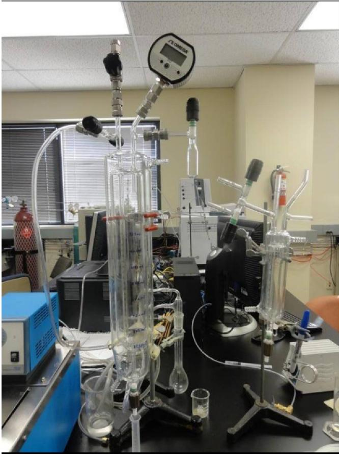
Figure 6.18: Photo of degassing glass apparatus in BEG gas geochemistry laboratory.
