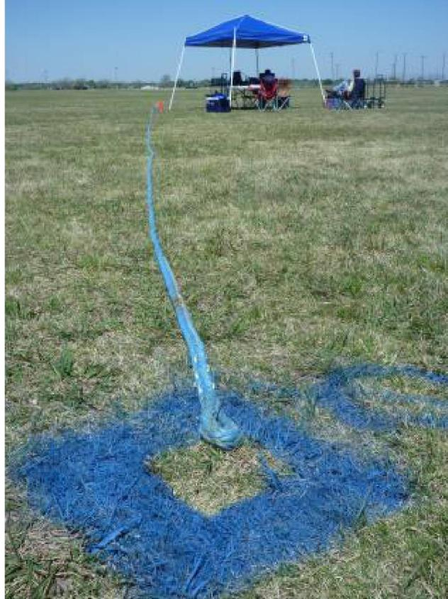
**Figure 8.9: Static field test using the cross cable. A series of tests were conducted to verify the accuracy of algorithms used to calculate streamer receiver position during the San Luis Pass dataset acquisition in July 2012.**
