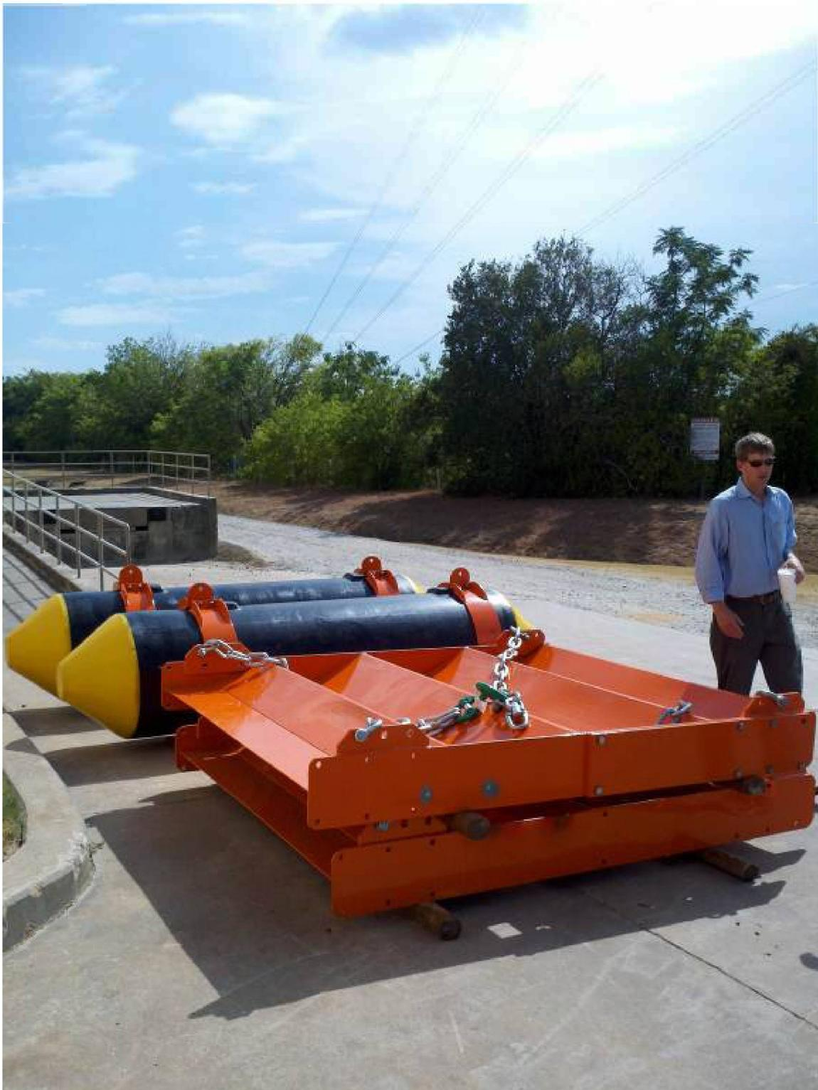
Figure 8.2: Photo showing the starboard and port paravane doors immediately after delivery at the Bureau of Economic Geology receiving dock. Tip Meckel on the right for scale.
