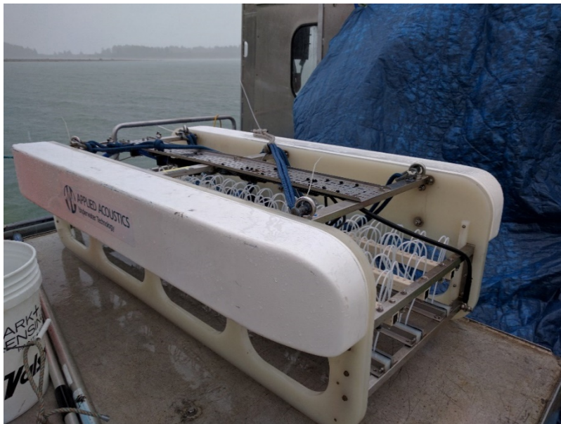
Figure 6. The Dura-Spark on top of the fish hold aboard the R/V Alaskan Gyre during the 2016 cruise (photo by Maureen LeVoor Walton, 2016).
