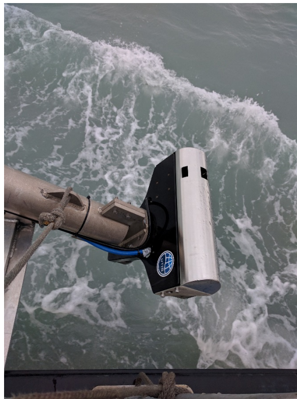
Figure 10. Two views of the assembled Reson multibeam unit and custom multibeam arm aboard the R/V Alaskan Gyre during a transit in 2016 (photos by Maureen LeVoor Walton). For acquisition, the arm settles into a cradle mounted just below the lab on the port side of the ship.
