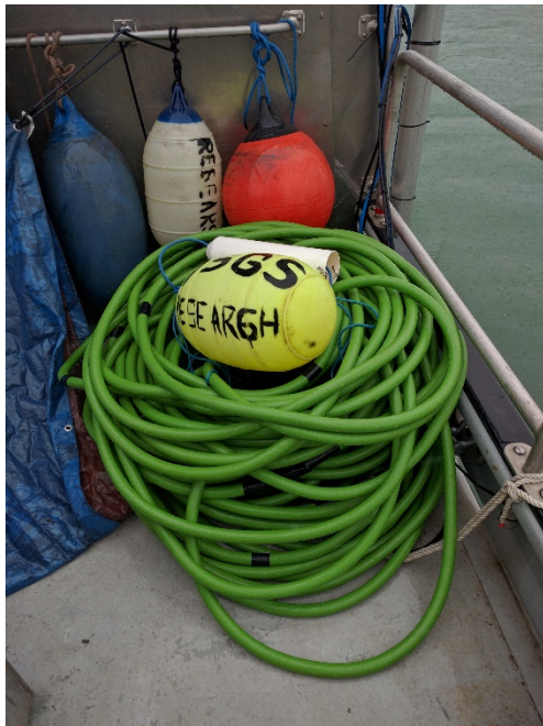
Figure 8 (left). TAMU MicroEel streamer on the deck of the Alaskan Gyre . Photo by Maureen LeVoor Walton (2016).
