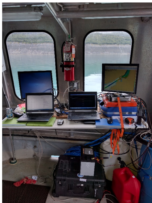
Figure 3. Lab setup during the 2016 Icy Bay/Taan cruise aboard the R/V Alaskan Gyre . Left: seismic. Below: multibeam. Photos by Maureen LeVoor Walton (2016).
