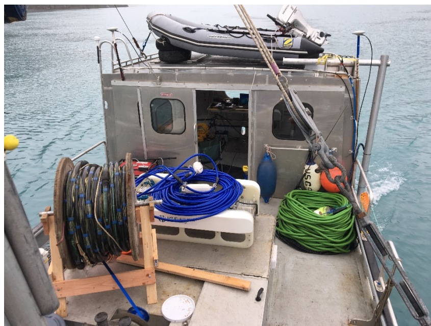
Figure 12 (left). Image looking aft of the Alaskan Gyre deck during acquisition. Three of the four GPS units used during acquisition can be seen mounted on the roof of the lab. The two Applanix units (flatter disks, longer poles) are located on opposite sides of the lab. The UTIG seismic GPS is mounted on the front of the starboard side ladder. The TAMU seismic GPS (not pictured) was mounted on the rear rung of that same starboard side ladder.
