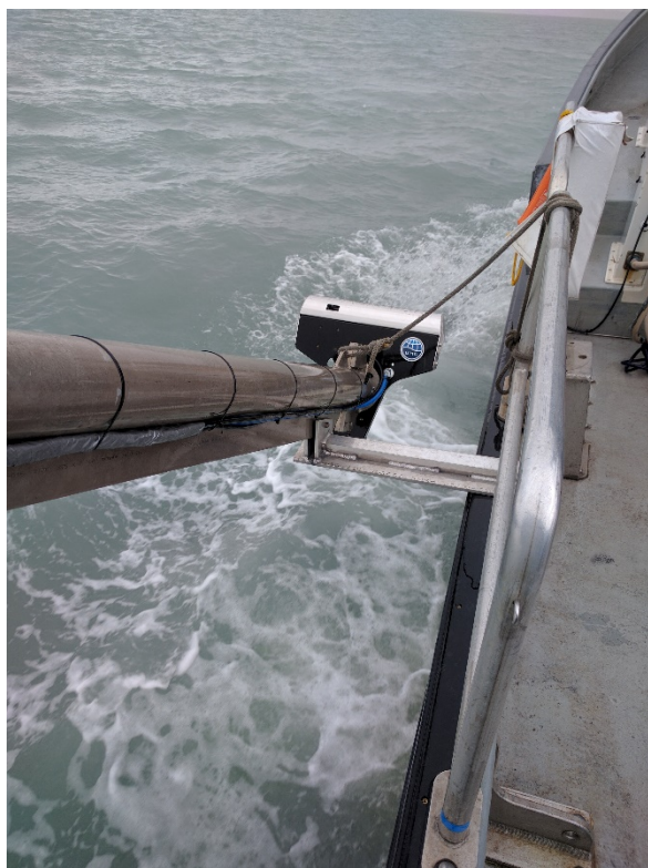
Figure 10. Two views of the assembled Reson multibeam unit and custom multibeam arm aboard the R/V Alaskan Gyre during a transit in 2016 (photos by Maureen LeVoor Walton). For acquisition, the arm settles into a cradle mounted just below the lab on the port side of the ship.
