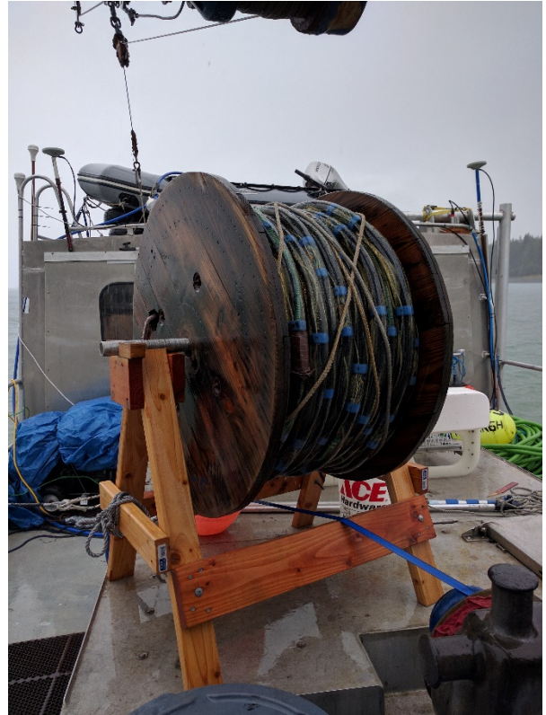
Figure 7 (right). Photo of the UTIG streamer aboard the R/V Alaskan Gyre during the 2016 cruise (photo by Maureen LeVoor Walton, 2016).
