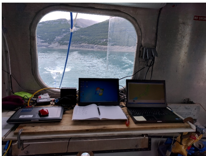
Figure 3. Lab setup during the 2016 Icy Bay/Taan cruise aboard the R/V Alaskan Gyre . Left: seismic. Below: multibeam. Photos by Maureen LeVoor Walton (2016).
