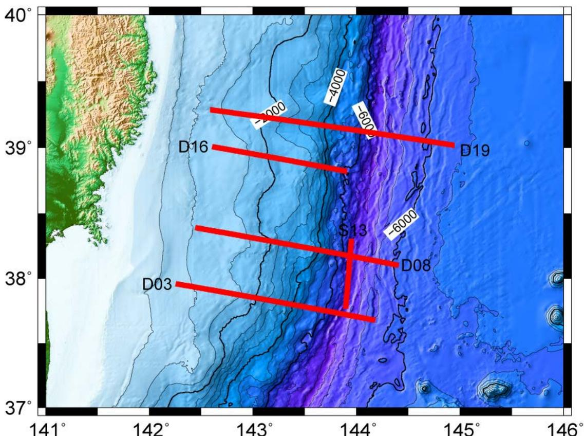
Red lines are MCS reflection survey lines conducted in this cruise using a tuned air-gun array and a 444 channel hydrophone streamer.
