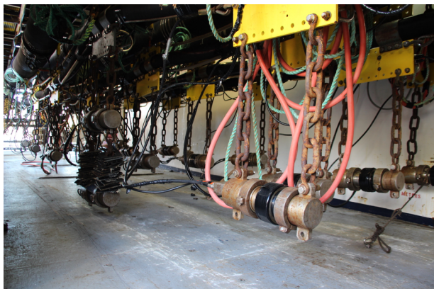
R/V Langseth 4-string, 36 element airgun array
