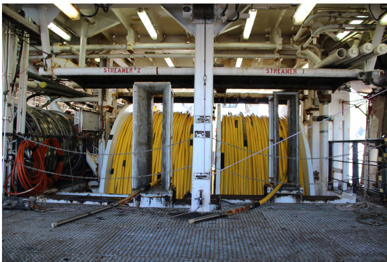
R/V Langseth solid-state streamer 1 and 2.
