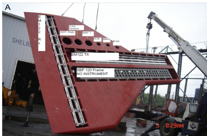
Figure A3.1. Bottom view of the Kongsberg EM122 transmit and receive arrays.
