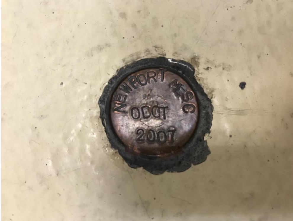
Figure 22. Gravity tie station. Gravity Value: g = 980\,595.99 mgals
