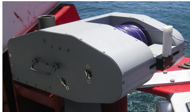
Figure 25b. Winch with automatic levelwind.
