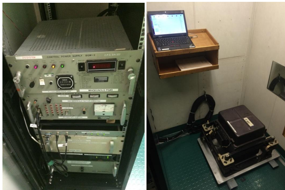
Figure 58. BGM3 electronics modules (left) and gyro-stabilized sensor platform (right) mounted in the NBP's gravity closet. The BGM3 was a last-minute replacement for the Lacoste and Romberg air-sea marine gravimeter that suffered serious problems prior to the cruise.
