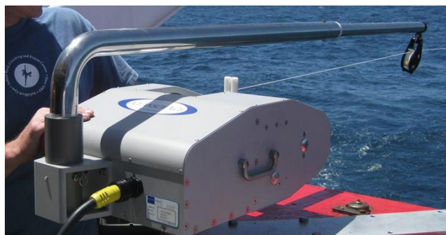
Figure 25c. Computer-controlled and semi-automated rewriter of tail spool.
