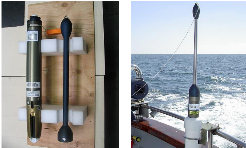
Figure 25a. CTD probe assembly: disconnected probe and tail spool components (left), and ready for deployment (right).
