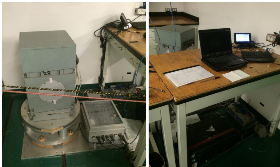
Figure 59. GT2M gravimeter mounted in the NBP's biology lab (left). The gravimeter is the tall stack of electronics mounted on the circular vibration isolation system and its power electronics are contained in the case to the right of the gravimeter. recording and real time monitoring is done with the two computers displayed to a small monitor and keyboard (right)
