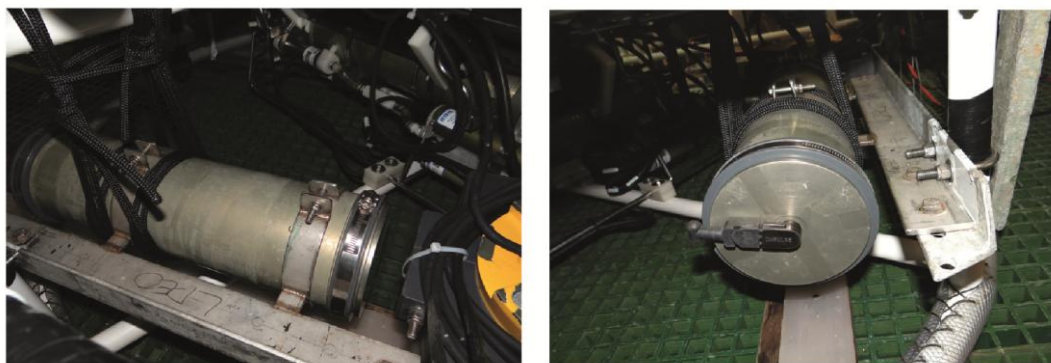
Figure 39. LDEO pressure housing for the IMP.
