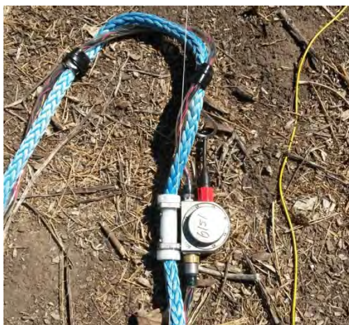
Figure 12 - Close-up of compass junction box aligned along control azimuth
