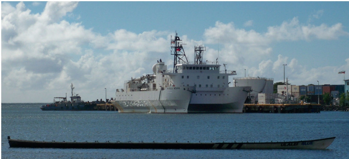
Figure 1.2: The R/V Kilo Moana in Apia, Western Samoa, in 2010. The Kilo Moana is a SWATH (Small Water Area Twin Hull) vessel owned by the U.S. Navy and operated by the University of Hawai‘i.
