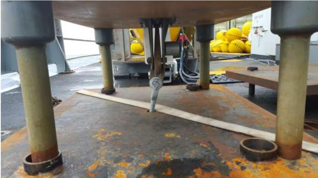
**Figure 4.5.1** BPR anchor plate.
