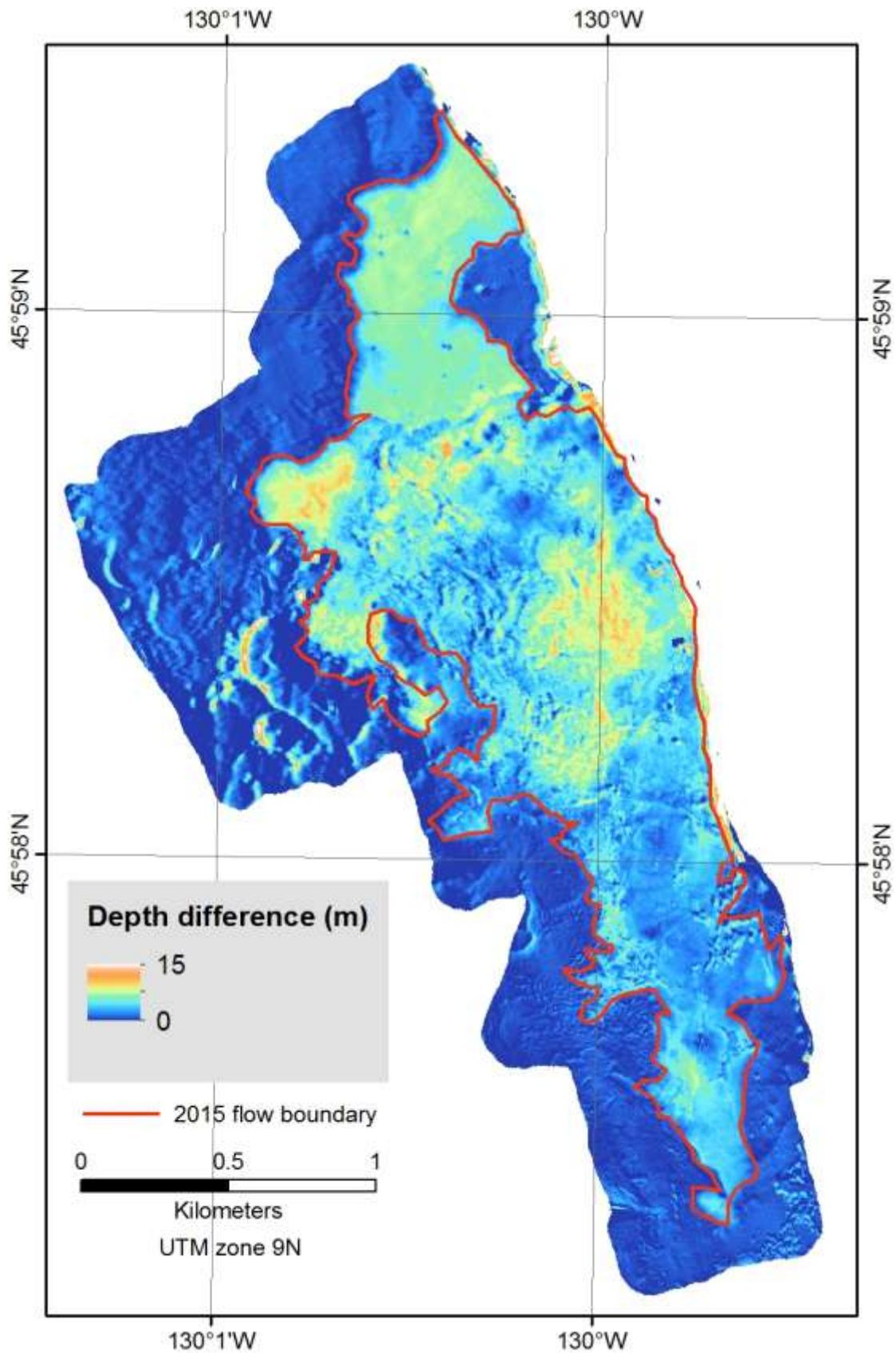
**Fig. 4.6.1-4** Map of bathymetric depth differences between 2015 AUV Sentry data and a compilation of MBARI's AUV data collected through 2011. Difference data was used to construct the 2015 flow boundary line depicted in red.
