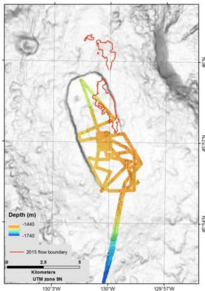
**Fig. 4.6.1-2** Map of bathymetry data from AUV *Sentry* survey 339, superimposed on a slope map of regional bathymetry. Boundaries of lava flows erupted in 2015 are shown (red lines) for reference. Map shown at the same scale as 4.6.1-3.
