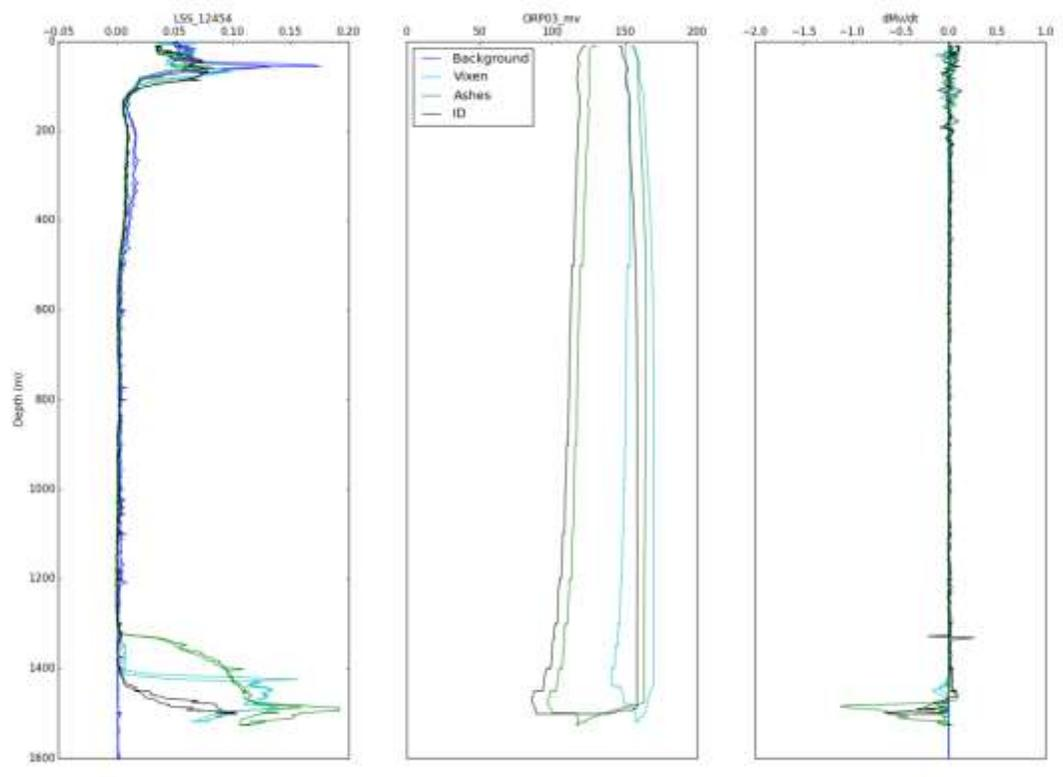
**Figure 4.4-5** LSS, ORP, and the time differential of ORP (dmV/dt) plotted with depth for vertical casts V15A01 (Background), V15A02 (Vixen), V15A03 (Ashes), V15A04 (International District Vent Field).
