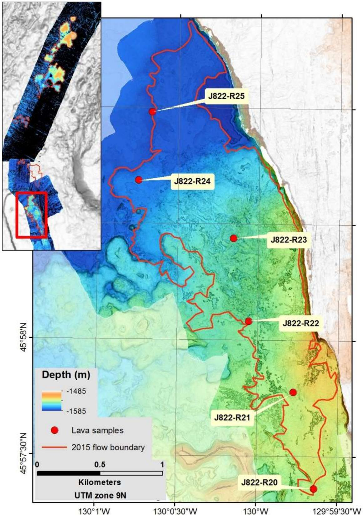
**Figure 4.2.1-** Map showing lava sample collection locations from ROV *Jason* dive J2-822 on the northeastern caldera floor of Axial Seamount. Bathymetry data from AUV *Sentry* survey 338 is superimposed over MBARI AUV data collected in prior years, both at 1 m resolution. Flow boundaries and inset map as described for Figure 4.2.1-1.
