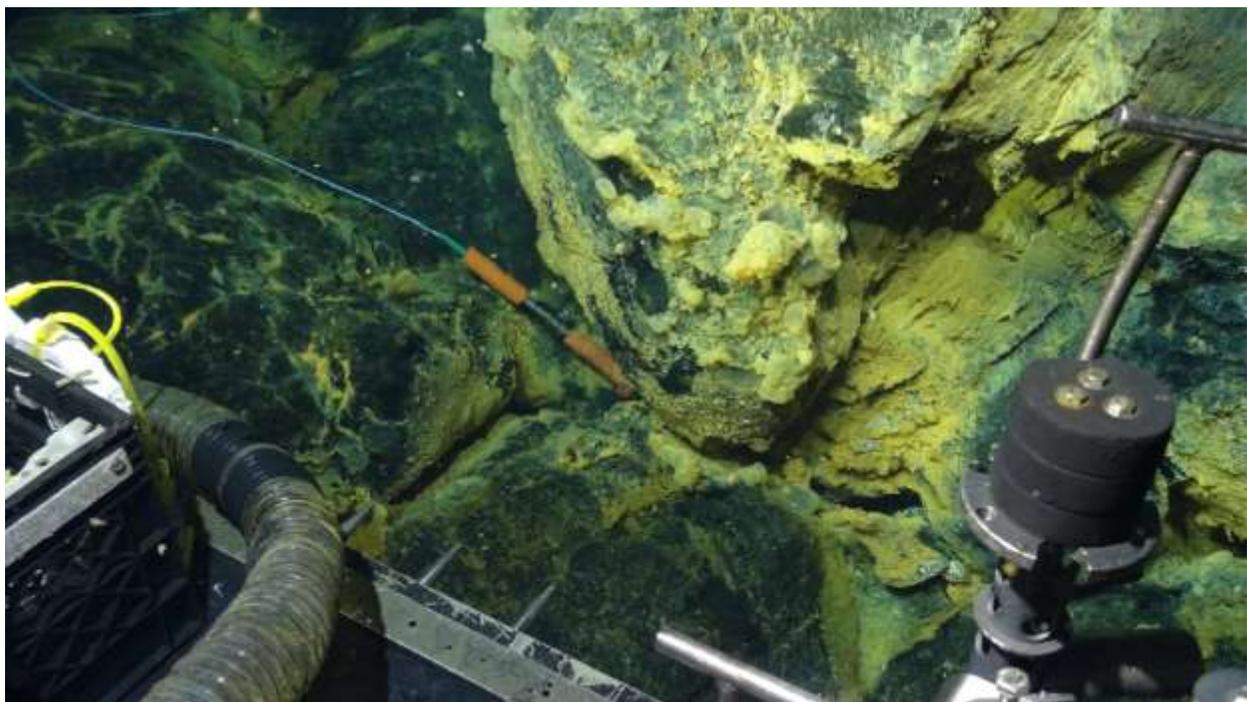
**Figure 4.2-7** Low-T vent with orange microbial mat and mucopolysaccharides globules on NRZ new lava flow. RAS intake with temperature recorder installed in crevice, where temperature was 19-20C.
