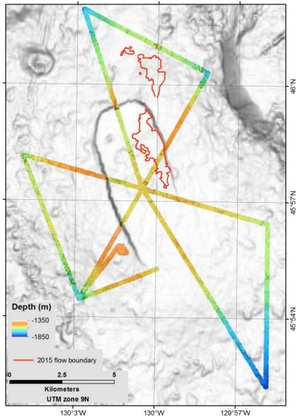
**Fig. 4.6.1-3** Map of bathymetry data from AUV Sentry survey 340, superimposed on a slope map of regional bathymetry. Boundaries of lava flows erupted in 2015 are shown (red lines) for reference. Map shown at the same scale as 4.6.1-2.
