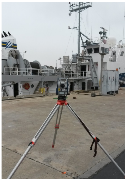
Figure 3 - Total Station over Monument SD1.
