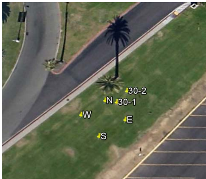
Figure 10. – Aerial view of baselines established for compass calibrations and verifications.
