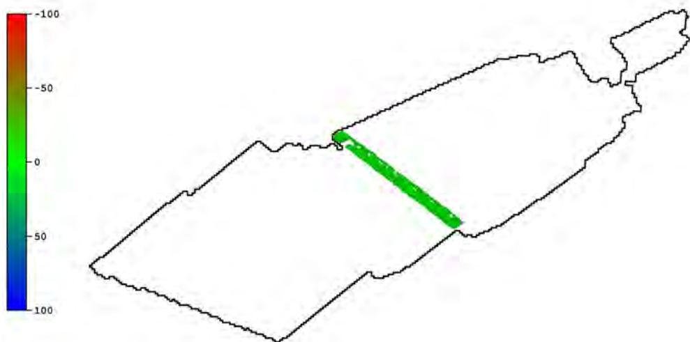
Figure 20: Surface difference between main-scheme and cross lines from leg 8, with survey outline. The differences range from -54m to 45m, with mean -0.3m and standard deviation 4.7m.
