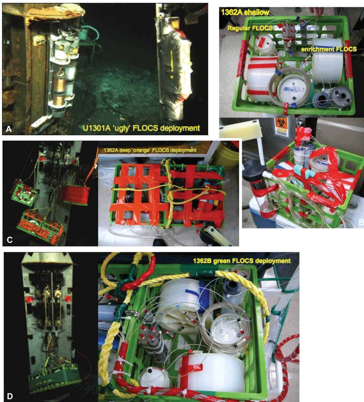
Figure 14. Deployment of FLOCS microbiology growth substrate during AT18-07. A. "Ugly" FLOCS system being installed on wellhead at Hole U1301A. B. New style FLOCS crate assembled in the lab for deployment to monitor shallow interval from Hole U1362A. C. Shallow FLOCS crate on left of wellhead, deep FLOCS crate hanging in center. Right image shows deep crate in lab prior to deployment. D. FLOCS crate hanging from wellhead in Hole U1362B, with umbilical leading to flowmeter bay. Right image shows crate in lab prior to deployment.
