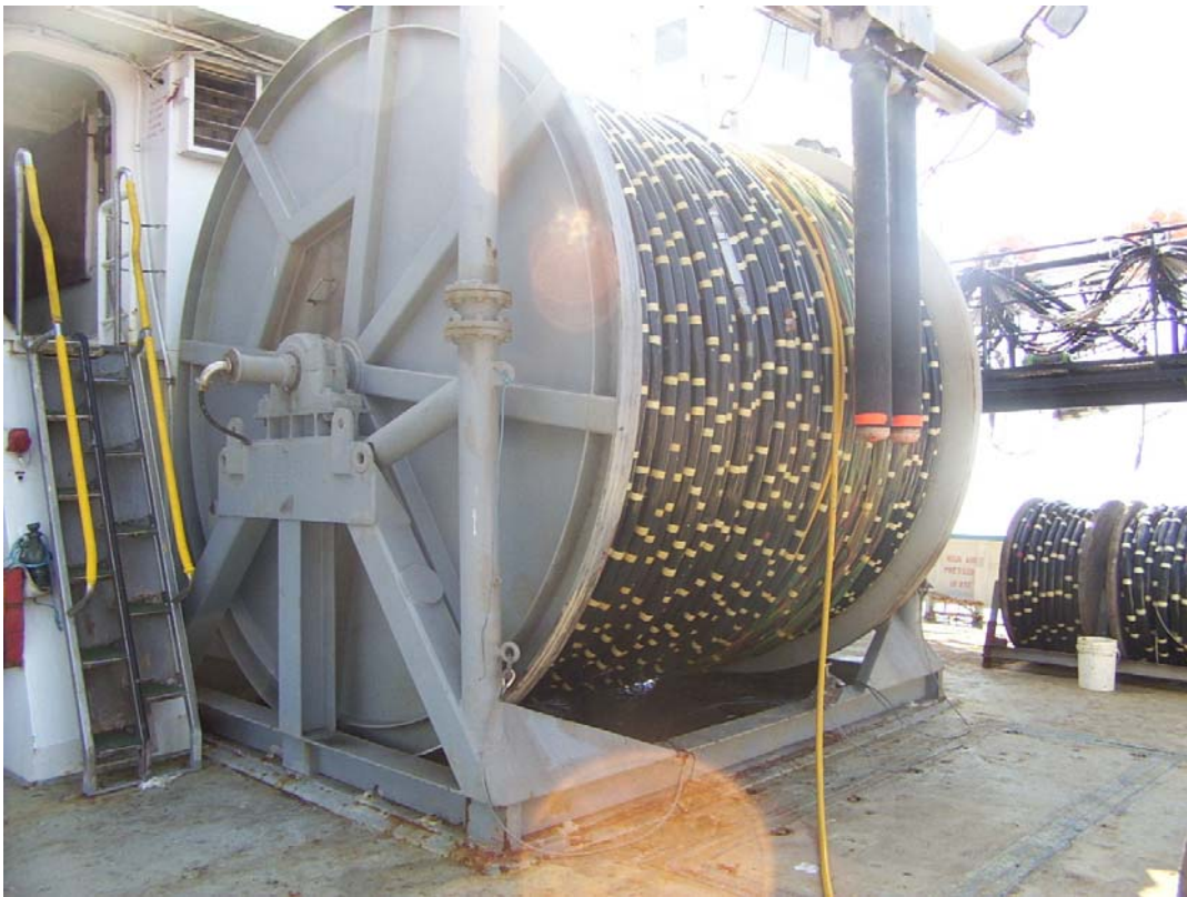
Figure 10. The Ewing 's 480 channel hydrophone streamer on the reel on the fantail. Replacement sections can be seen in the background and digitizing cans can be seen spaced along the streamer (these sum the acoustic signals and send them up the streamer to the recording systems on the vessel).
