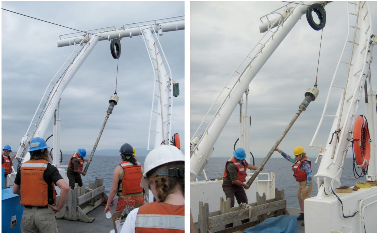
Fig. 43. Gravity corer being retrieved with the A-frame winch.
