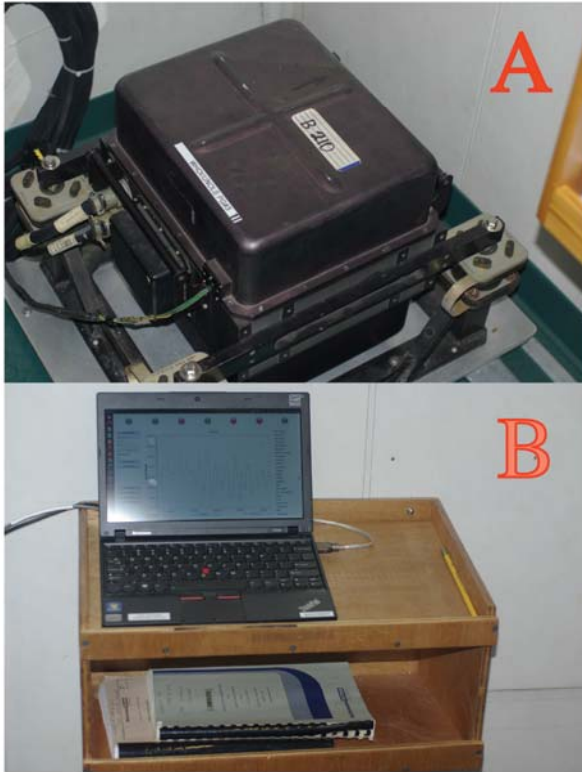
Fig. 5a-1A View looking down on BGM3 gravimeter Serial number S210, showing gimble mount.
