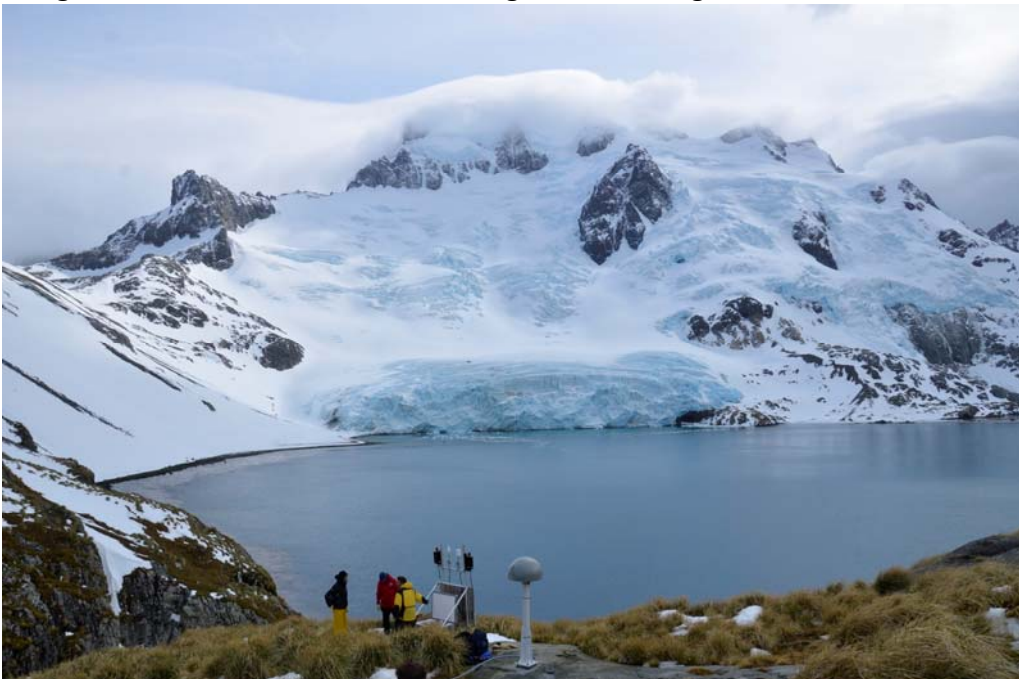
Fig. 6.2 GPS “frame” containing the electronics (GPS receiver, iridium modem, power controllers), solar panels, wind generators, weather station and iridium antenna) foreground, GPS antenna and mounting mast in background. View ~SE.
