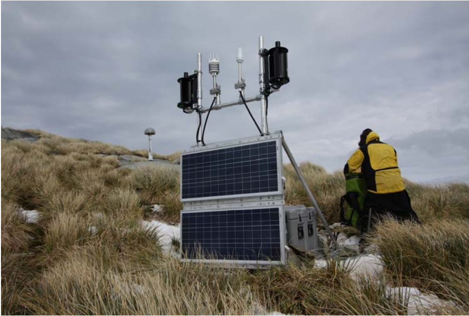
Fig. 6.2 GPS “frame” containing the electronics (GPS receiver, iridium modem, power controllers), solar panels, wind generators, weather station and iridium antenna) foreground, GPS antenna and mounting mast in background. View ~SE.
