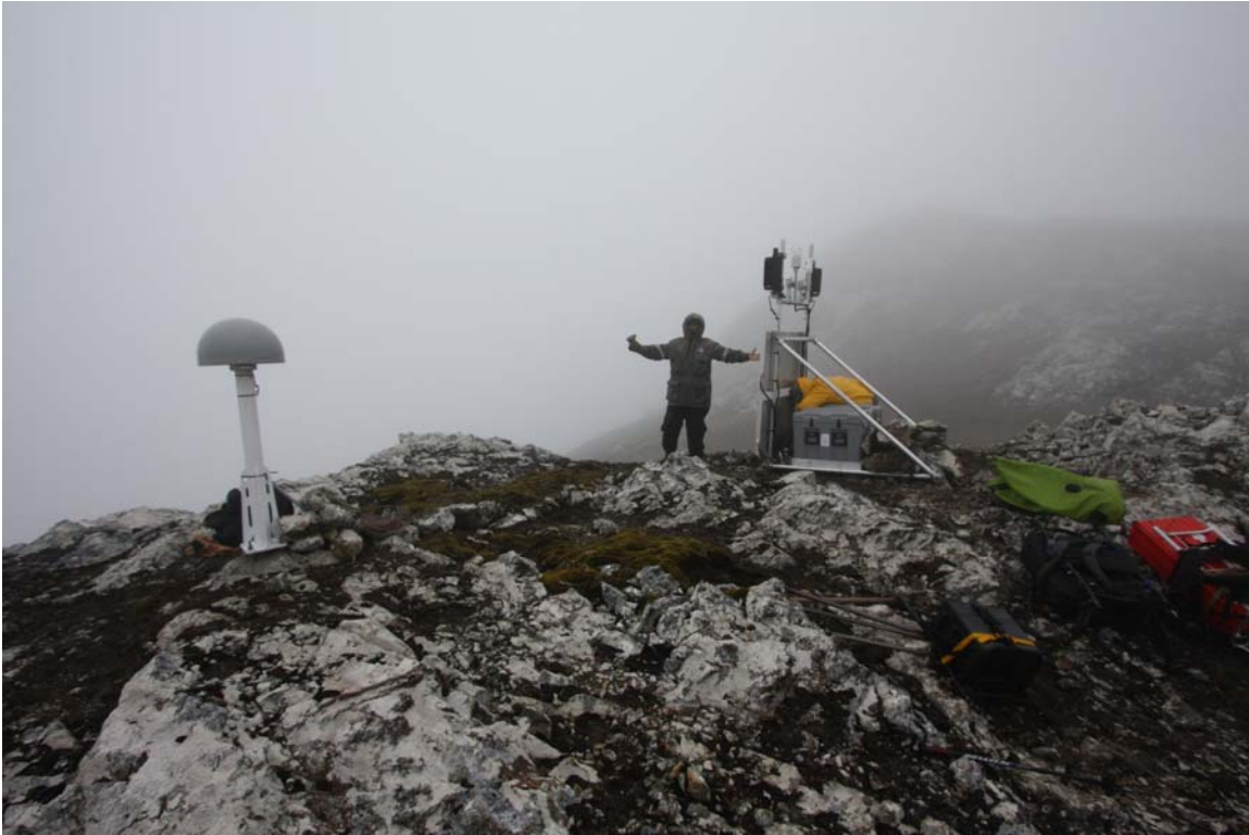
Fig. 6.5 View ~ ENE of site SGO2 showing GPS antenna and mast and GPS frame.
