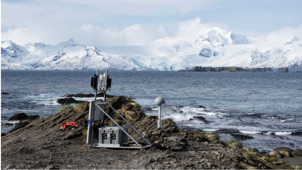
Fig. 6.7. View slightly N of E showing GPS frame, antenna and mast of SGO3. Small area of tussock behind site.
