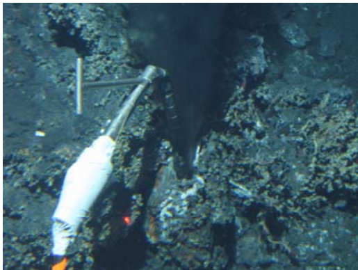
Figure 2.5.3. Insertion of the resistivity probe into a black smoker orifice at Dante vent.
