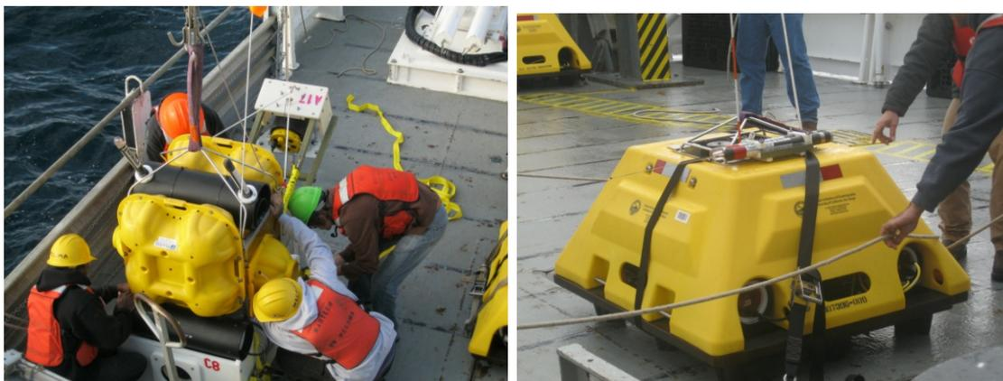
**Fig 2:** Left SIO Abalone Ocean Bottom Seismometer. Right LDEO seismometer, pressure sensor, hydrophone instrument package.
