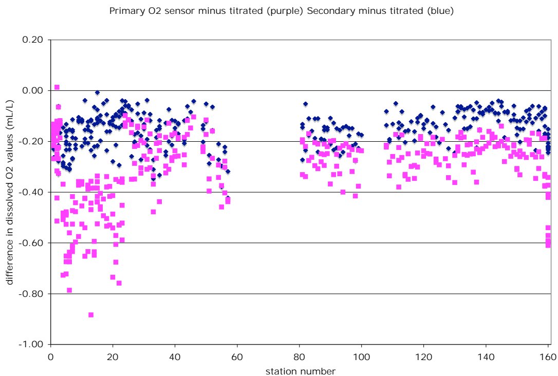
Figure 6: Ox1 minus Ox2 sensor values versus CTD station number. Note significant errors between CTD stations 4 to 23, and 160.
