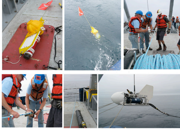
Figure 6: Photos of the towed array deployment. From left to right: stray-line buoy with float and acoustic transponder, stray-line buoy in water, attaching electrodes and feeding out the array (next two), Bunyip recorder in case with syntactic foam and SBL transponder attached, and lastly, the SUESI deployment.
