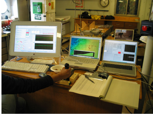
Figure 2: Control console for SUESI's Labview interface showing vital signs and flight height, with winch controller, Fledermaus visualization of depth profile, and acoustic navigation (also controlled by LabView).
